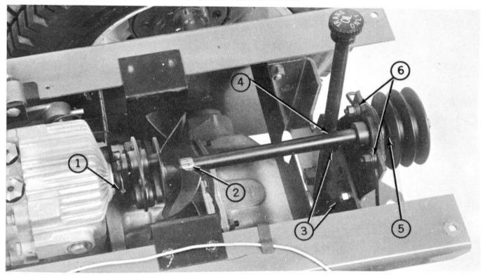
Remove fender deck and upper fan housing. Remove and discard fan.
