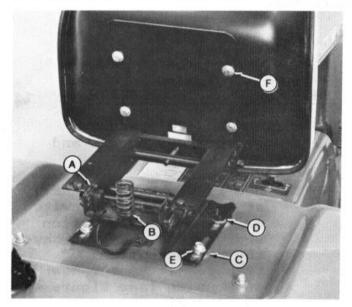
NOTE: Suspension shown here is on a new 430 Tractor (Serial # 475001 and up) equipped with new style seat switch (A) and spring (B). If your tractor has this new switch, it must be transfered to the new suspension as shown.
