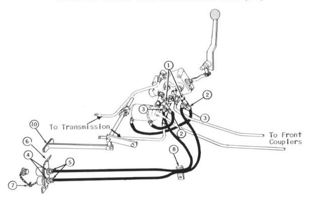
Disconnect cylinder oil hoses from tee fittings on control valve.
