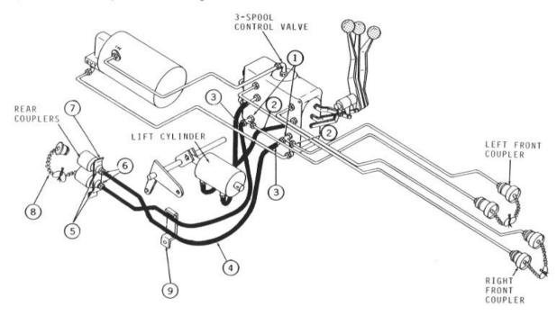
Remove two left front hydraulic lines from lower elbows on control valve.
