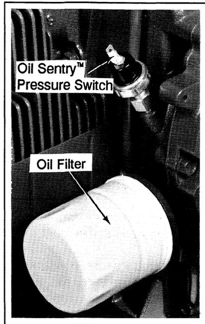
Figure 6. Oil Filter and Optional Oil Sentry™ Switch.
