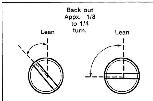
Figure 11. Optimum Main Fuel Setting.
