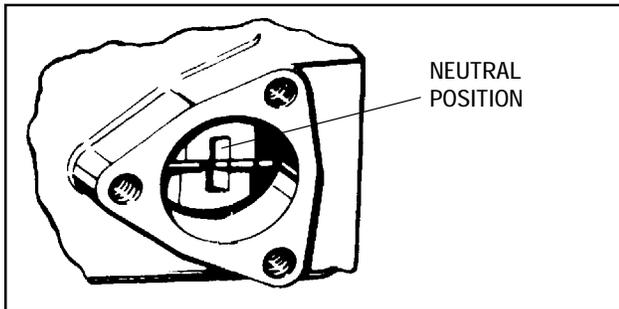
1. Clean the outside surface of the transaxle, away from the area where disassembly will take place. Position shift lever in neutral position to help disassembly. Remove screws (3) holding shift lever. Remove all keys from keyways, remove all burrs and dirt from shafts. On hardened shafts, use a stone to remove burrs. All seals should be replaced whenever a shaft is pulled through a seal. Always use a new gasket whenever the gasket surfaces have been separated.
