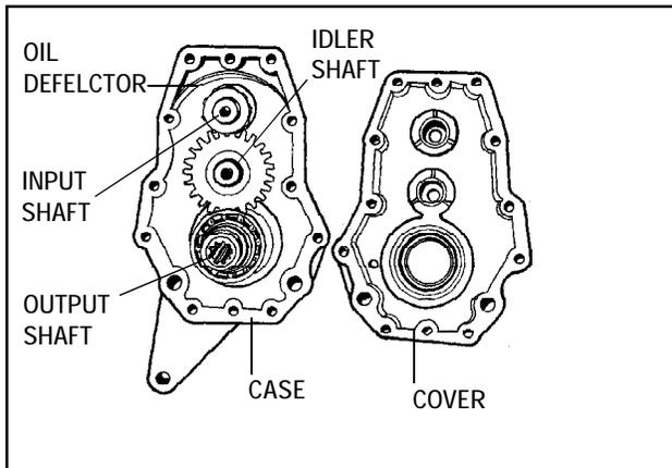
5. Before closing case and cover together, inspect to make sure all parts are present. Now place new gasket between case and cover.
