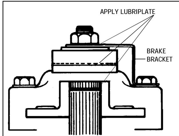
9. Prior to installing the brake assembly, apply a light film of lubriplate to the inside of lever portion which contact pins, also to outside of lever which contacts flat washer and between shaft O.D. and bore of brake disc. Brake pads and brake disc must be free of grease and oil. Install brake assembly.
