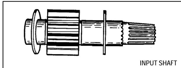
7. Remove the input shaft and two washers. The input shaft and gear are one piece.
