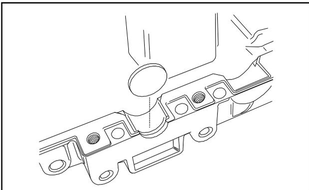
11. To seal the case and cover at the end of the shifter/brake shaft, a flat plug is placed there (end opposite the brake assembly). Clean the mating surfaces of case and cover; place a continuous thin bead of sealant all around the seam. Use Loctite Gasket Eliminator #515, Tecumseh part number 510334 or the Loctite Silicone RTV 598, Tecumseh part number 788093. Install cover screws and torque to 90-100 inch pounds.
