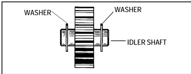
3. Place idler gear into case with washers on both sides along with output shaft at the same time.
