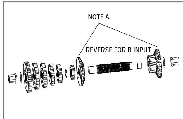
8. To disassemble the counter spur gear shaft, remove the bushing, thrust washer and spur gears (or spacers if used) the last spur gear is held in place by a retaining ring. Remove the retaining ring and slide the spur gear and forward drive bevel gear off the splined end of the shaft. The bushing, thrust washer and reverse drive bevel gear can be removed from the unsplined end of the shaft.
