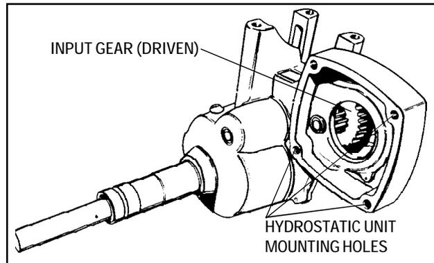
2. After removing the hydrostatic unit, inspect the surfaces and the gears from outside unit.
