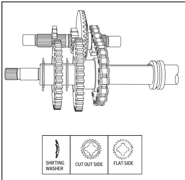
5. Build the gears on the countershaft and shifter/brake shaft alternately, meshing each gear with its mating gear on the other shaft. The first gear on the shifter/brake shaft would be the largest of the shifting gears. Place this gear next to the neutral collar with the flat side of the gear next to the collar.
