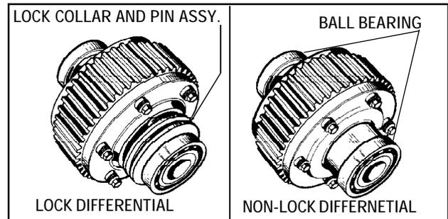
3. Check differential lock collar for fork slop or pin wear.
