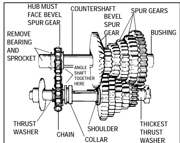
1. Remove gear and shaft assemblies from case half of the transmission by lifting the two shafts out of the bearing supports taking care not to disturb drive chain relationship with sprockets.
