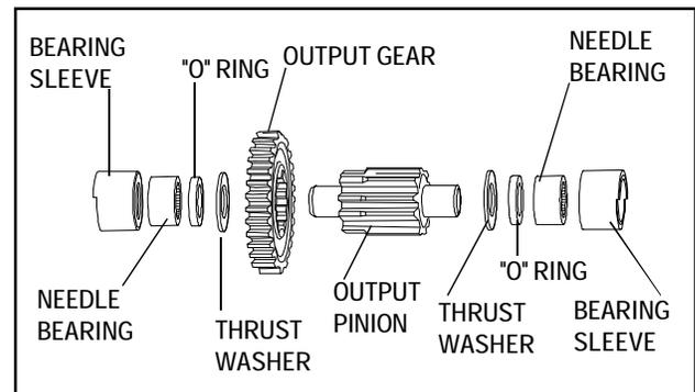
5. **OUTPUT PINION AND SHAFT.**
