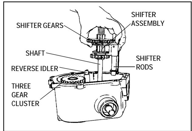
7. Remove complete shifter assembly by grasping shifting gears, shaft and both shifter rods as a unit.
