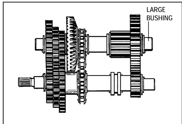
6. Then place a thrust washer on each end of the countershaft and a bushing on the end with the largest gear.
