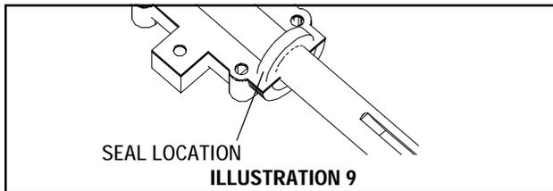
Pick up the entire assembly and place it into the case positioning the seals in the seal pocket. When properly installed the axle shaft should turn freely without any binding. (Illustration 9)
