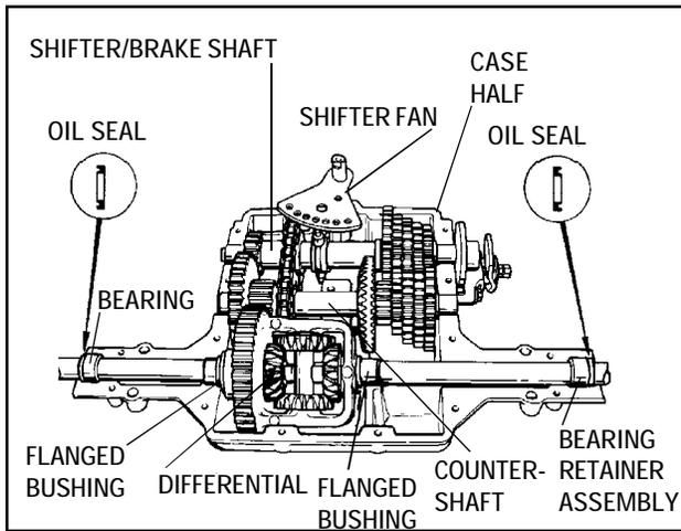
4. Remove gear and shaft assemblies from case half by lifting the two shafts out of the bearing supports taking care not to disturb drive chain relationship with hubs on sprockets.
