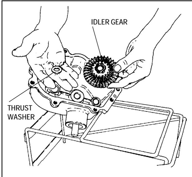
1. Underneath the idler gear is one (1) washer in stead of a thrust bearing and two (2) thrust washers.
