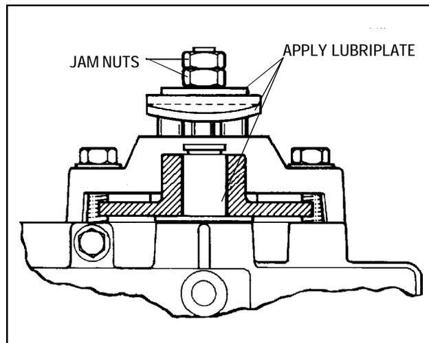
When assembling, apply a light film of lubriplate to the inside lever portion which contacts the pins, also to outside of lever, which contacts flat washer, and between shaft O.D. and bore of brake disc. Brake pads and brake disc must be free of grease and oil.
