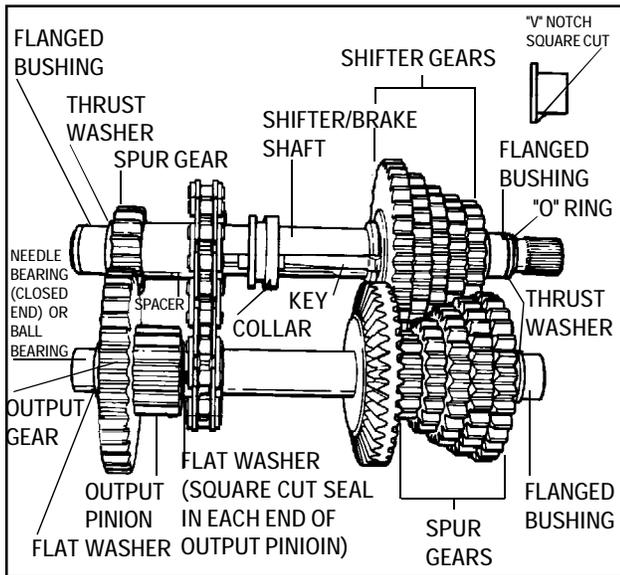
8. Install the output and pinion gears, the flat washer, square cut rings, needle bearing (closed end), and spacer on one end and thrust washer and flanged bushing on the other end. Note that the "V" notch on the bushing fits into recess "V" in case.
