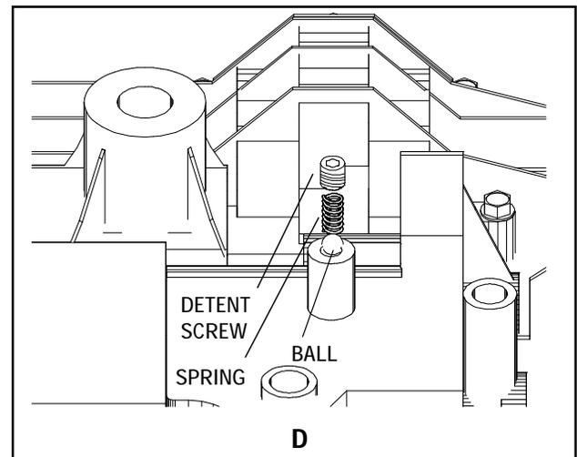
6. Remove the set screw, spring and index ball (See Illustration D).
