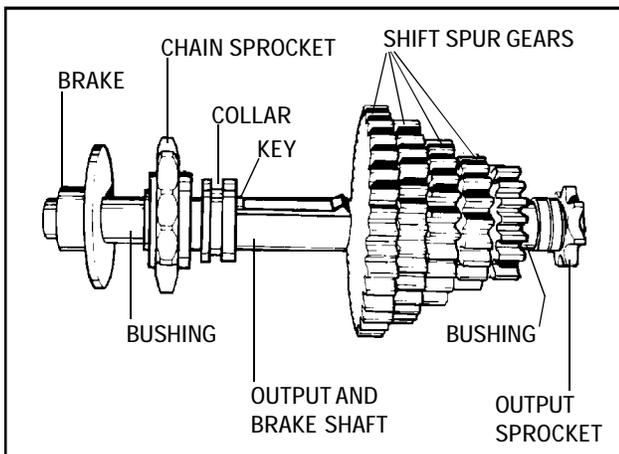
3. Remove the output sprocket and brake disc from the output shaft. Remove the bushings, shift spur gears, chain sprocket, collar and keys.
