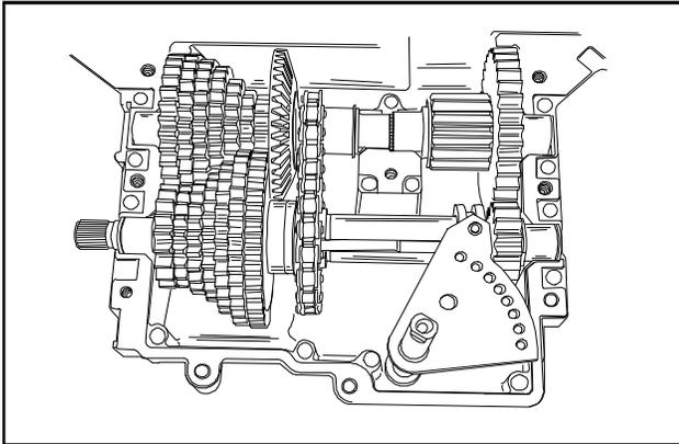
10. Install the shifter assembly and bearing strap, pack the transaxle with the remaining Bentonite grease (30 ounces total). Apply grease to top of shift fan.
