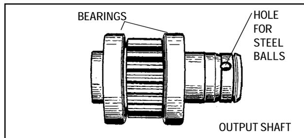
8. Remove output shaft. Output shaft bearings can be removed by using a bearing splitter and puller.
