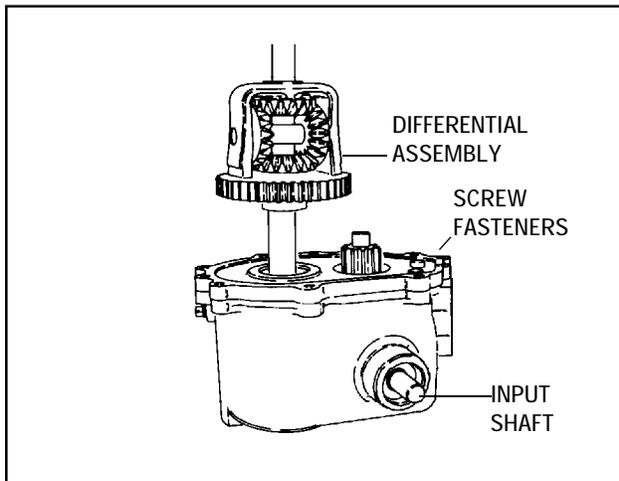
5. To remove differential assembly, it may be necessary to replace two or three screws to hold center plate assembly down. Pull assembly straight up. If tight, tap on lower axle with soft mallet. **CAUTION: DO NOT USE STEEL HAMMER.** Refer to the chapter on differential assembly service. Remove gear on top of shifter shaft.
