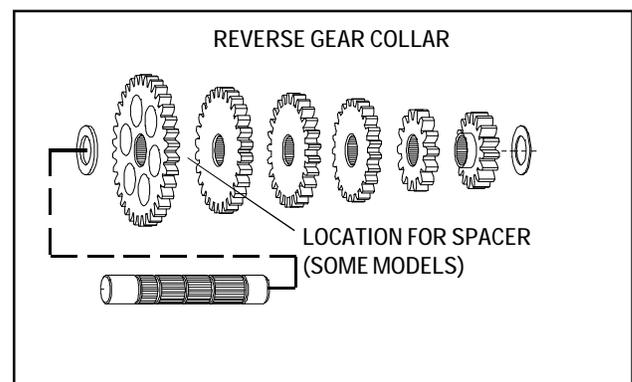
5. The countershaft must have the longer unsplined end toward the outside or brake side of the case and the shorter unsplined end toward the shifter assembly. The wide washer or spacer is placed on the longer unsplined end followed by the largest spur gear.
