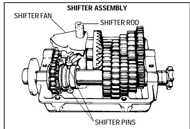
3. Remove cover. Remove shifter assembly (includes shafts, pins and fan from transmission by lifting shaft out of case).
