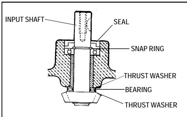
3. The input shaft has one (1) thrust washer only, instead of a thrust bearing and two (2) thrust washers.
