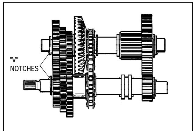
4. Remove gear and shaft assemblies from case half. **NOTE:** Before disassembly, observe how "V" notches on the flange bushings fit into recess "V" of case.
