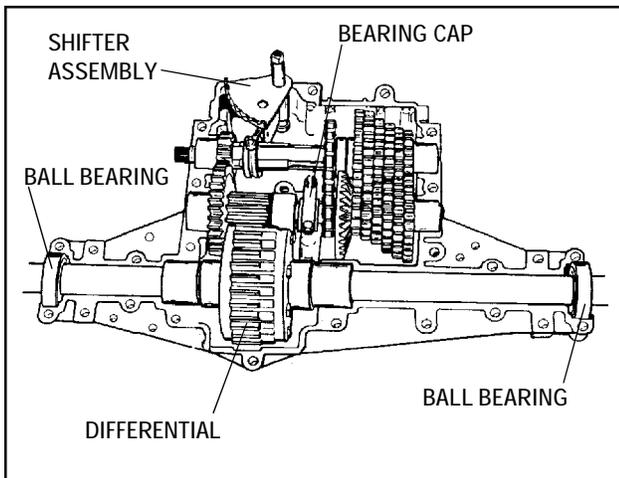
9. Insert differential into case, position the caged ball bearings on the axle ends into the recessed areas of the case. Place the bearing cap over the sleeved needle bearing of the countershaft and torque bolts 90-100 inch pounds. Install shift fan and pack transaxle with remaining Bentonite grease. (36 oz. total)
