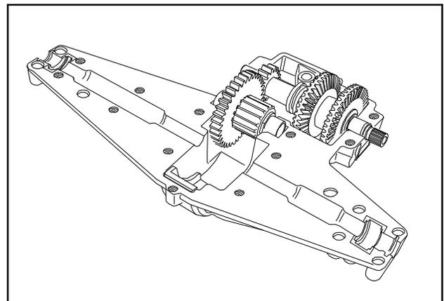
5. Remove the top bearing block on the bull gear of the differential. Remove the bull gear, bevel pinion gears with center shaft and the axles.
