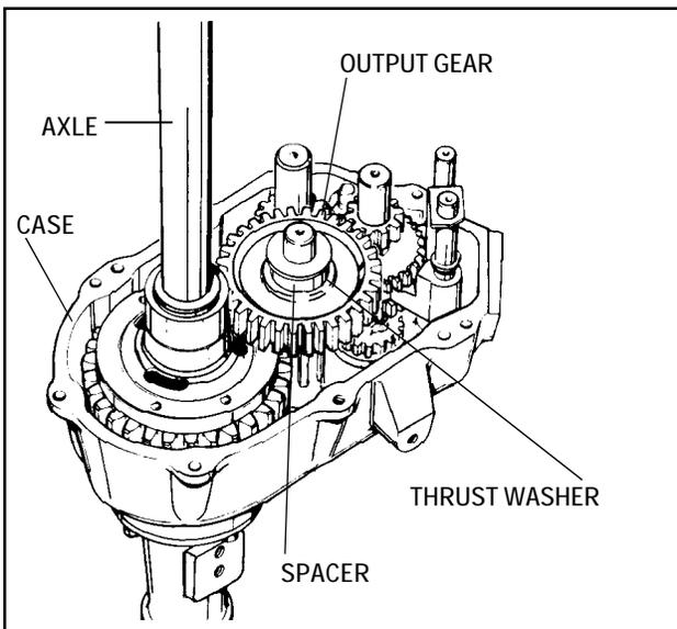
6. Install the output shaft, gear, spacer and thrust washer.
