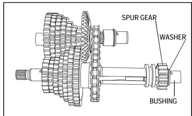
7. Place the spur gear onto the splines on the other end of the shifter/brake shaft. The thin washer and bushing conclude the assembly of these 2 shafts.
