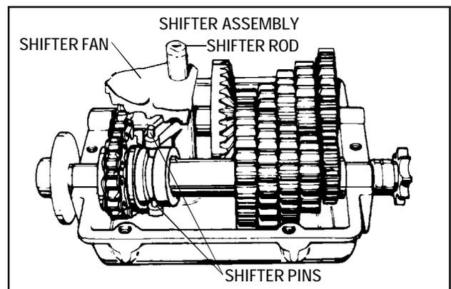
8. Install shifter assembly (shaft, pins and fan) 12 oz. Bentonite grease around gearing, and reinstall cover on case. Torque cap screws 90-110 in. lbs.
