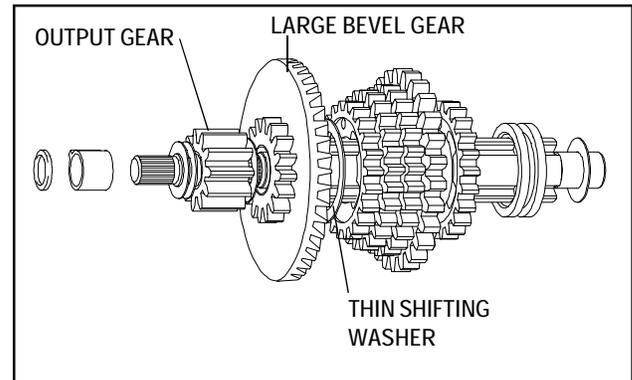
4. The last shifting washer will be a thin flat washer installed prior to the large bevel gear. The style of input will determine how the large bevel gear will be installed. In the model pictured input "A" is used and the bevel is inward towards the keys. On models with a "B" input the bevel will be outward or away from the keys.
