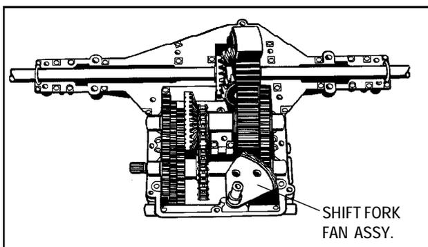
13. Install shifter assembly and pack 26 oz. Bentonite grease around bearings, gearing, and top of shift fan then reinstall cover on case. Torque cap screws 90-100 inch pounds.
