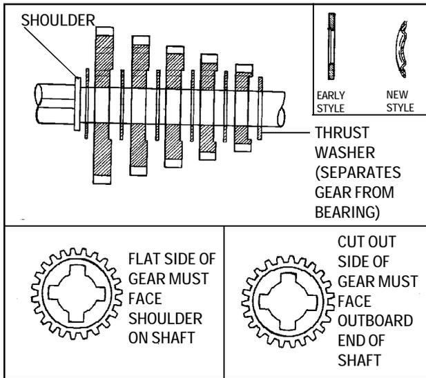
3. Install the thrust washers and shifting gears onto the shifter/brake shaft. The number of gears and/or spacers will be determined by the number of speeds in the transmission.
