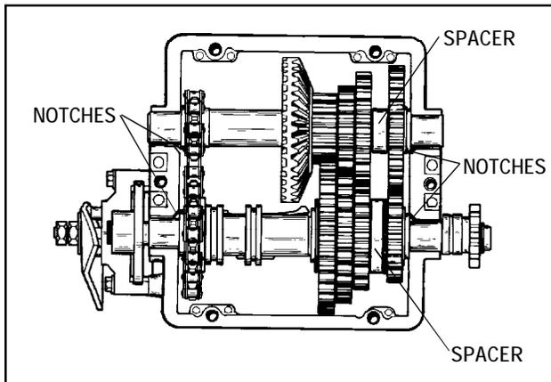
Install bronze bearings and disc and sprocket. Install shaft assemblies into case utilizing piloting locators on bearings to properly align notches in case. **CAUTION:** Be sure bearing locators are seated in transmission case.
