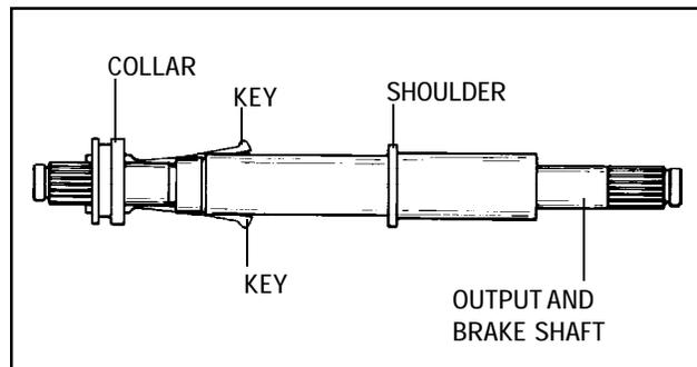
2. Install collar and keys on output shaft. Thick side of collar **MUST** face shoulder on shaft.
