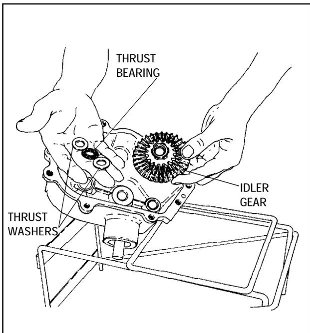
11. Remove the idler gear, thrust washers and thrust bearing.
