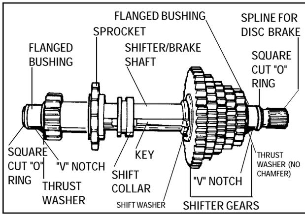
4. **NOTE:** The thrust washer on the shift gear end, of the shifter and brake shaft, does not have a chamfer on the inside diameter. Install sprocket, spacer, spur gear, and thrust washer on output shaft. Be sure collar on sprocket faces the shift collar. Install bushings on both ends of shifter/brake shaft, install square cut "O" rings on end of flanged bushings.
