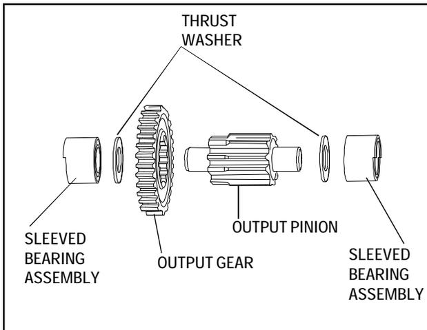
8. Place the output gear on the stepped end of the output pinion. Place thrust washers on each end and then the large sleeved needle bearings. Install the three shaft assemblies into the case.
