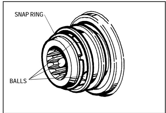
9. Install 3 steel balls in holes with a little grease to hold them in place.
