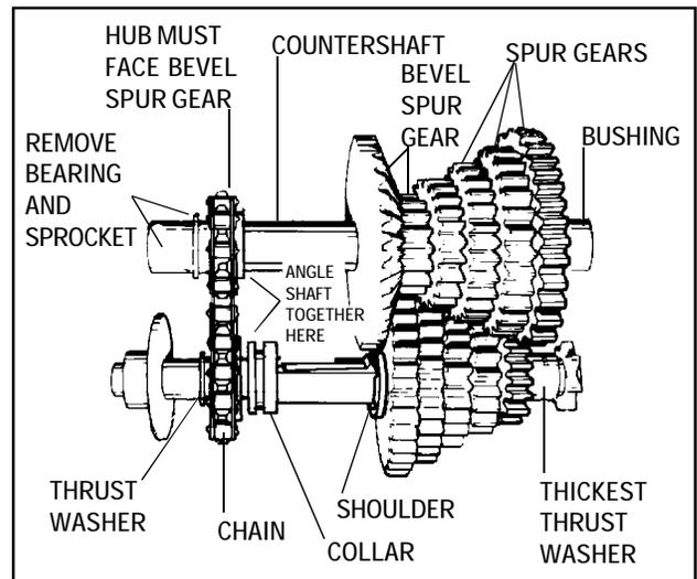
6. Install chain over two shafts registering chain on output shaft sprocket and in-line with serrations on countershaft. Be sure collar on sprocket faces shifting keys and collar.
