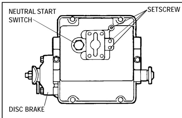
If installed, (optional equipment), remove neutral start switch.
