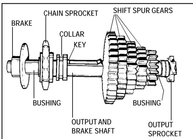
4. When correctly assembled the output shaft should appear as shown.
