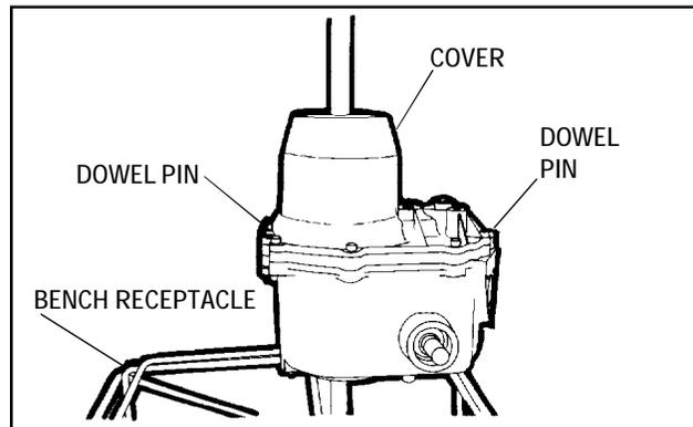
3. Remove the socket head cap screws holding the case and cover together. Drive out the dowel pins used for alignment of the case and cover.
