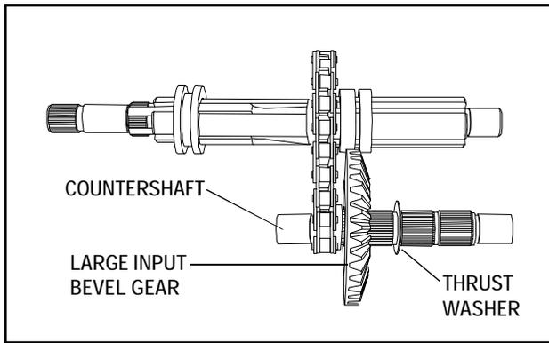
4. Insert the countershaft into the smaller reverse sprocket. Then install the large bevel gear, with the bevel facing away from the reverse sprocket. Place thin thrust washer on the countershaft next to the bevel gear.
