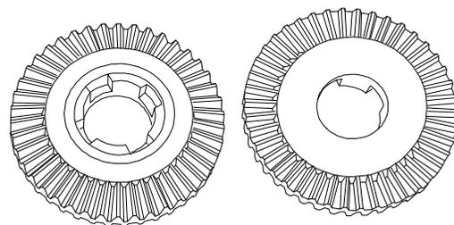
3. The large beveled shifting gears can be placed onto the shifter/brake shaft. The bevels on the gears face each other and are separated with a neutral spacer. Push shifting keys into the neutral spacer.
