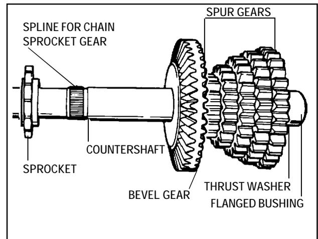
7. Remove the sprocket, bevel gear, spur gears, thrust washer, and flanged bushing. The spur gears are splined to the countershaft.
