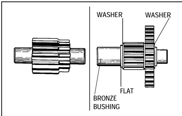
9. To assemble the output shaft assembly, place a washer and then the bronze bushing with collar, (flat down), next to the pinion. Place output gear over pinion as in picture. There is a washer on outside of gear.
