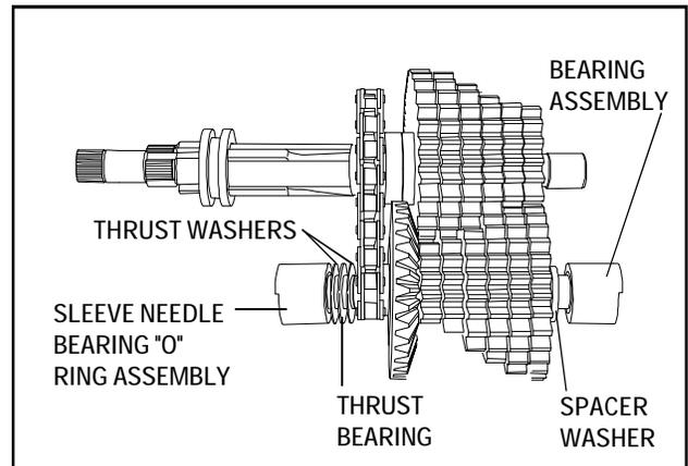
6. In the model pictured, a thrust washer, thrust bearing, thrust washer and sleeved needle bearing with "O" ring are placed on the countershaft next to the reverse sprocket. Place a spacer washer and sleeved needle bearing with "O" ring next to largest spur gear. The sleeved needle bearing installation will have the step facing outward and the wider portion of the bearing sleeve toward the cover. This will be true for all future sleeve bearing installations.
