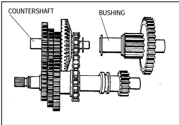
5. To disassemble countershaft, output pinion and shaft assembly, simply pull apart.
