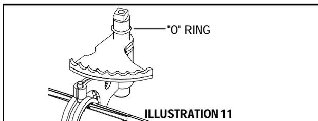
Before placing the cover on the case, place the shift rod and fork pins into the shift collar and shaft into the boss in the case. Inspect the shaft on the rod and fork for rust and burrs. (Illustration 11)
