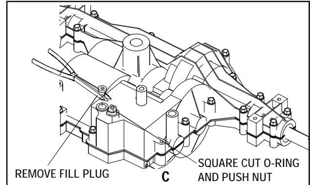
3. Remove the oil drain / fill plug located on top of the unit. This can be done by using a needle nose pliers to pull the plug out. Drain all of the oil from the unit. (See Illustration C)
