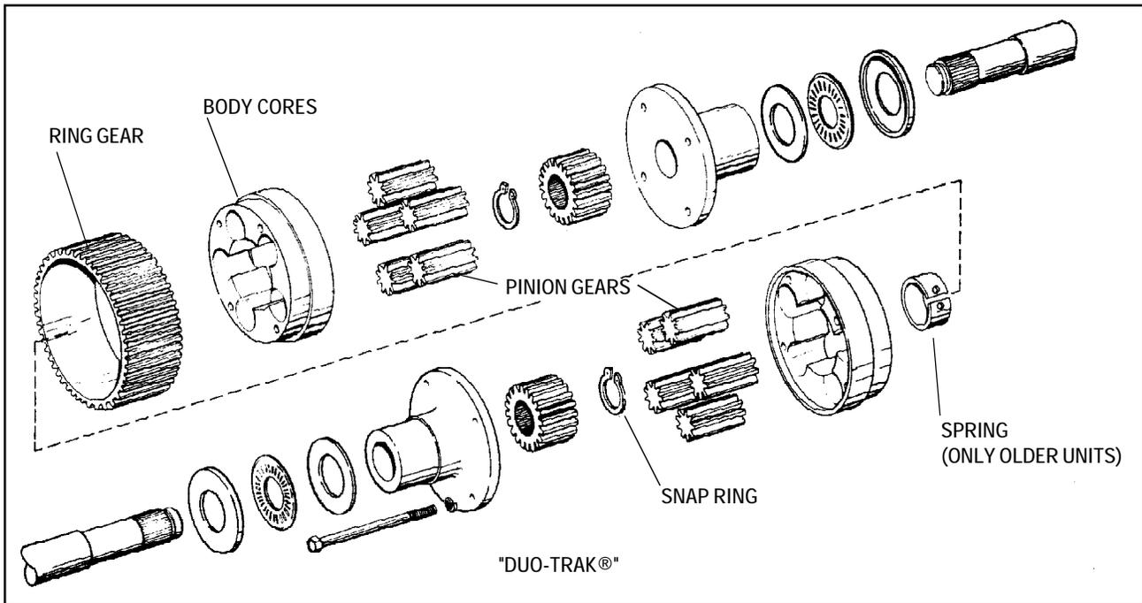
\*DUO-TRAK is the trademark of a patented limited slip differential designed by Illinois Tool Works.
