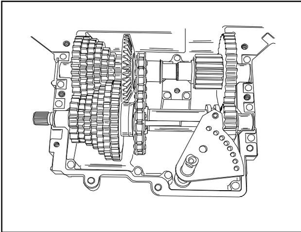
10. Install the shifter assembly and bearing strap, pack the transaxle with the remaining Bentonite grease (30 ounces total). Apply grease to top of shift fan.
