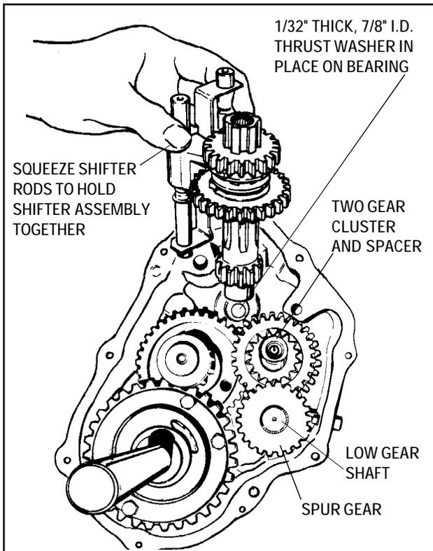
6. Install a 1/16" thick by 3/4" I.D. thrust washer, gear and low gear idler shaft in cover. Do not put a thrust washer on the exposed end of this shaft. Be sure the small gear meshes with the larger gear of the two gear cluster.
