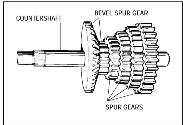
5. Install bevel spur gear and smallest to largest spur gears to the splined end of the countershaft.
