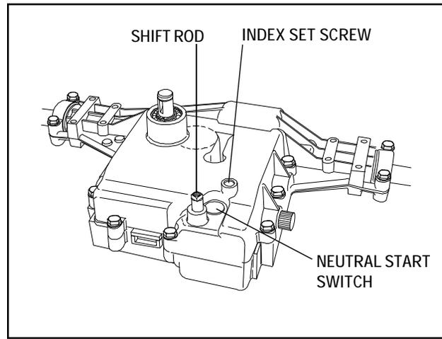
11. Guide cover over shift rod and position onto case. Torque cover screws 180-216 inch pounds. Replace index ball, spring and set screw and turn set screw one (1) turn below flush. Install the neutral start sensing switch if applicable. Check for binding by turning input shaft.
