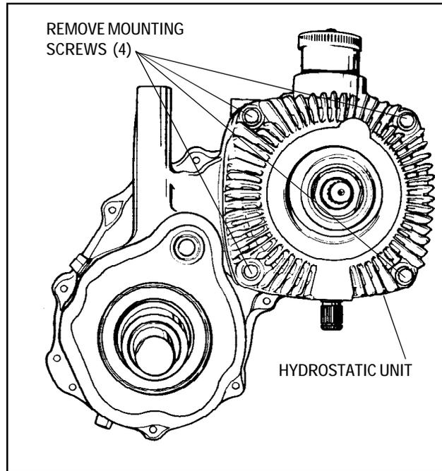
1. To separate the hydrostatic unit from the 1300, support both parts, then remove the four mounting screws, and separate the parts. Drain oil from the 1300 unit. Any hydrostatic repair must be done through the equipment brand dealer.
