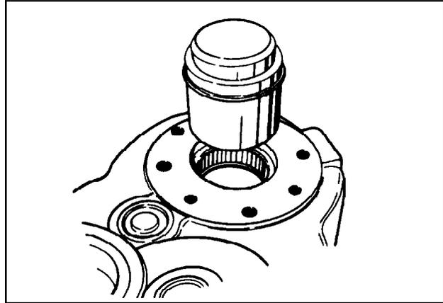
1. Use a bearing tool to press out the bearing. Insert the proper tool in the bearing, and with an arbor press, press out the bearing from the inside.
