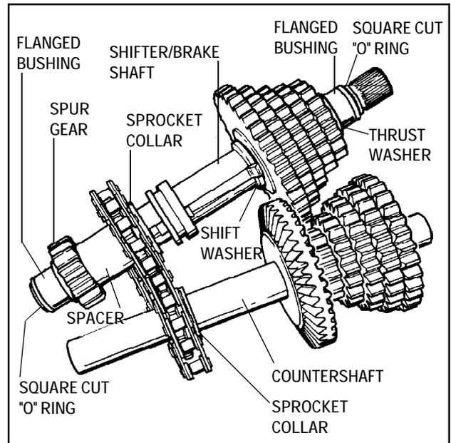
6. With the shifter/brake shaft and countershaft ends angled together, install the chain on the sprockets.
