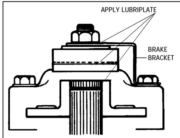
13. Prior to installing the brake assembly, apply a light film of lubriplate to the inside of lever portion which contact pins, also to outside of lever which contacts flat washer and between shaft O.D. and bore of brake disc. Brake pads and brake disc must be free of grease and oil. Install brake assembly.
