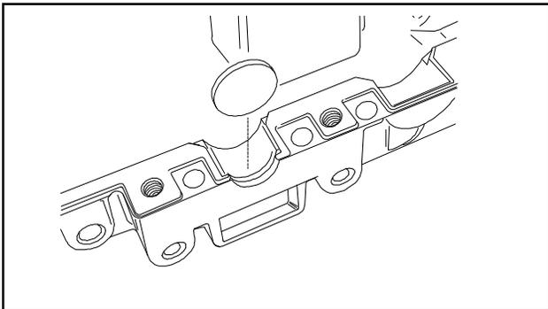
11. To seal the case and cover at the end of the shifter/brake shaft, a flat plug is placed there (end opposite the brake assembly). Clean the mating surfaces of case and cover; place a continuous thin bead of sealant all around the seam. Use Loctite Gasket Eliminator #515, Tecumseh part number 510334 or the Loctite Silicone RTV 598, Tecumseh part number 788093.
