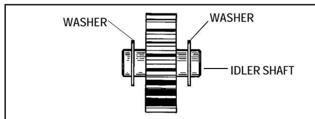
9. Remove the idler shaft and two washers.
