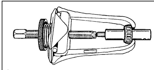
5. Remove shaft out of cage.\* Remove roller bearing with outside puller toward threaded side. Remove snap ring.
