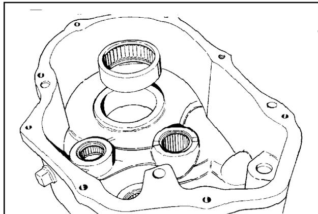
4. The inside face of the bearing housing should be below the thrust face on the case or cover. This distance is controlled by the design of the inserting tool. By using the proper tool, bearing life will be extended. Bearings should be pressed into the cover .015" to .020" below the thrust surface. The open end bearing in the low speed shaft of four speed transaxles, is to be .010" below the thrust surface. The open end bearing in the shifter shaft should be .010" below the end.
