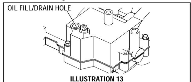
10. Refill the transaxle through the fill hole located in the cover. This unit requires 16 oz. of 80W90 gear lube (part #730229A). When completed lubricate the plug lightly on the outside with oil. Use a 3/16" wood dowel placed in the recess of plug and push it into the plug hole (Illustration 13).
