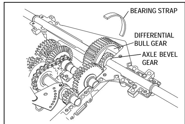
5. Remove the bearing strap on the bull gear of the differential. Some models do not use a bearing strap. Remove the bull gear, bevel pinion gears with center shaft and the axles. Grasp the axle bevel gears between your thumb and fingers, hold together while lifting differential from case.
