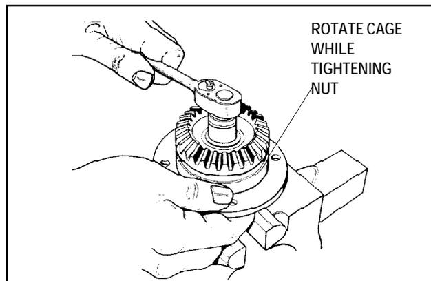
14. To achieve proper pre-load on bearings, place the outboard side of shaft in protected vice. Begin to tighten nut on gear side, while turning cage until a very slight drag is achieved on the cage housing with no end play. Parts must spin freely.
