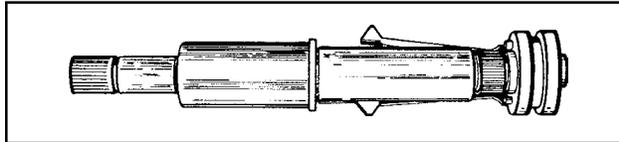
2. Grease both keyways and slide keys and collar on shifter/brake shaft.
