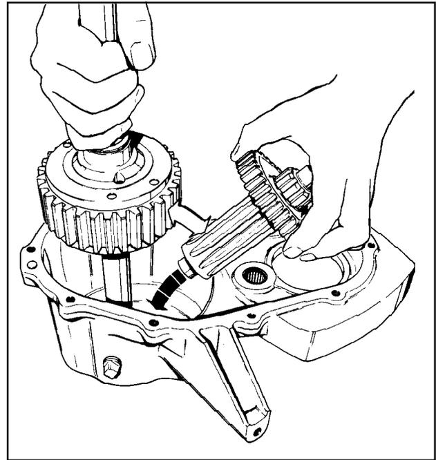
1. When installing axle support, be sure case and cover alignment is true with the press. Press support in until flanged surfaces contact case and cover.
