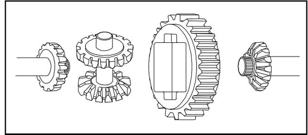
**NOTE:** The differential must be assembled out of the case and then placed in the case.
