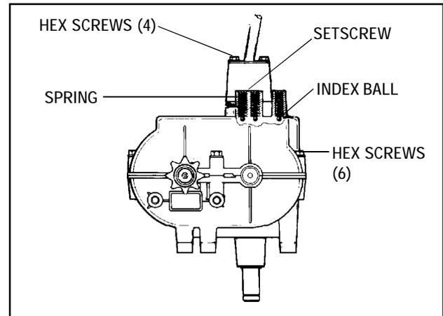
1. Remove shift lever by removing four hex screws on shift lever cover.
