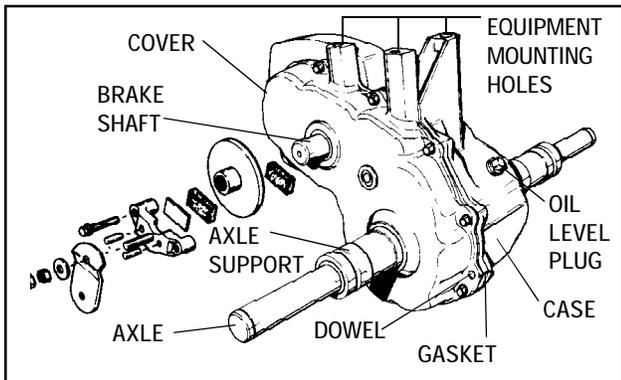
Axle supports, pressed from the inside out, must be removed with the case and cover, similar to the method used in the 1200 series transaxle.
