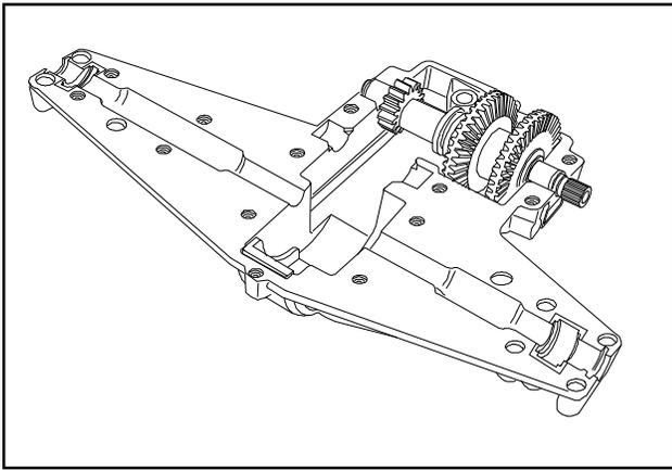
6. Remove the output shaft assembly.
