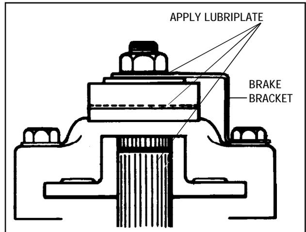
Apply a light film of lubriplate to the inside of lever portion which contacts pins, also to outside of lever which contacts flat washer and between shaft O.D. and bore of brake disc. Brake pads and brake disc must be free of grease and oil.
