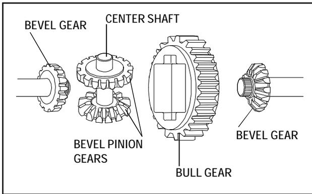
**NOTE:** The differential must be assembled out of the case and then placed in the case. Apply Bentonite grease to axle contact areas of case.
