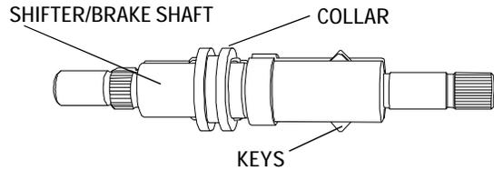
2. Grease both keyways and slide keys and collar on shifter/brake shaft.
