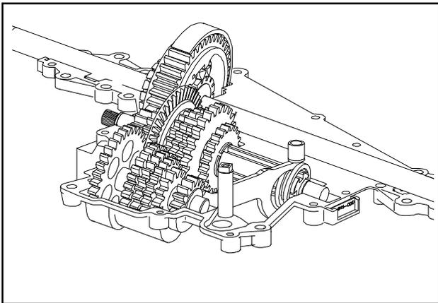
7. Install the shifter assembly, bearing strap and reverse idler assembly (if applicable). Pack the transaxle with the remaining Bentonite grease (10 ounces total). Replace index spring and ball.
