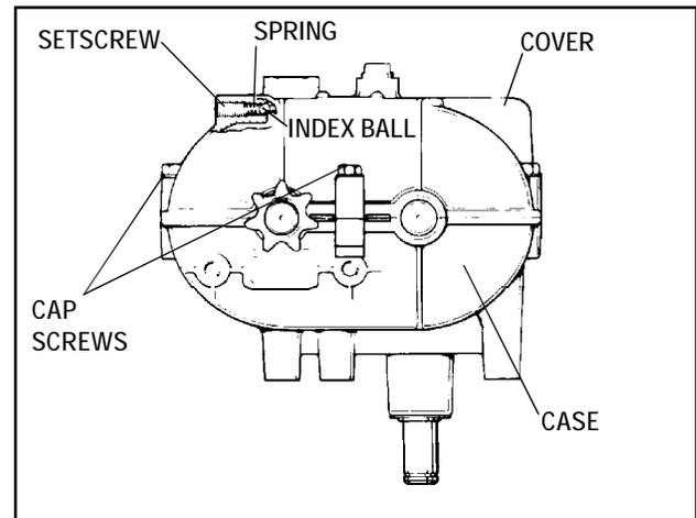
1. Remove setscrew, spring and index ball from transmission cover.
