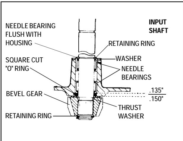
8. The input shaft can also be removed and inspected or serviced. Remove the snap ring on the bevel gear and pull the shaft through the case. The square cut "O" ring must be replaced if the shaft is removed.
