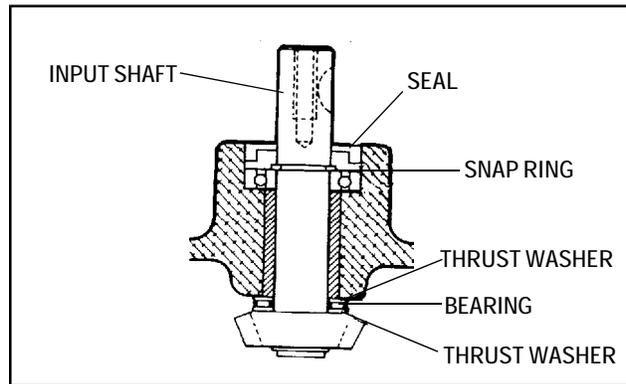
12. Remove input shaft oil seal to allow access to snap ring. Remove snap ring and input shaft will slide out. A removed seal must be replaced by a new seal.
