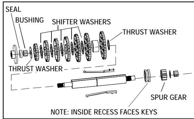
7. To disassemble the shifter/brake shaft, start on the spur gear side. Remove the oil seal, the bronze bushing and thrust washer. Remove all of the shifter spur gears (or spacers if used) and shift washers. Remove the neutral collar, reverse gear and thrust washer. On the output side of the shifter/brake shaft remove the bronze bushing, thrust washer, and output spur gear.
