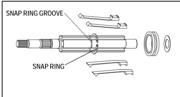
2. Grease all keyways and slide keys and collar onto the shifter/brake/output shaft. On models which have a inner diameter recess cut into one side of the shift collar, the recess side must face towards the gears and snap ring for proper gear selection. Place large snap ring back into the snap ring groove. On five speed models that do not use the large bevel gear for the highest speed an additional neutral spacer will be placed between the snap ring and the shift collar.
