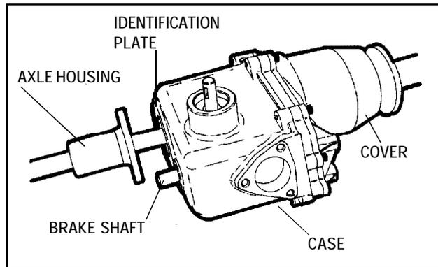
2. After removing axle housings, place the unit in a receptacle, bench or clamp the transaxle in a soft jaw vise. Position the transaxle so that the socket head cap screws are facing up.
