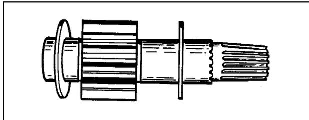
4. Place one input shaft washer on bearing boss next to idler gear. Place proper seal protector for input shaft in seal and insert shaft and second washer.
