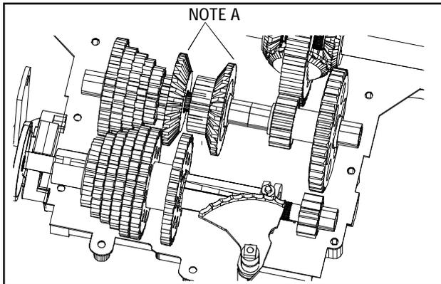
5. There are 3 shaft assemblies in this transaxle. The countershaft, shifter/brake shaft and output shaft. Remove shifter fork assembly and then remove these assemblies from the case.
