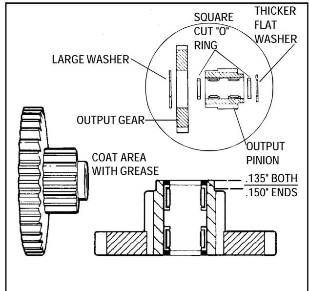
7. For correct positioning of the needle bearings use removal and installation Tool Part No. 670252. Fill the area between the needle bearings with grease before installing on the countershaft.
