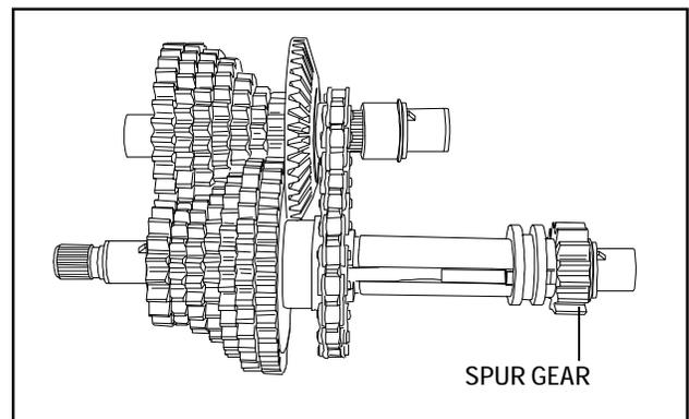
7. Place the spur gear onto the splines on the other end of the shifter/brake shaft. The thin washer, bushing, and "O" ring conclude the assembly of these 2 shafts.
