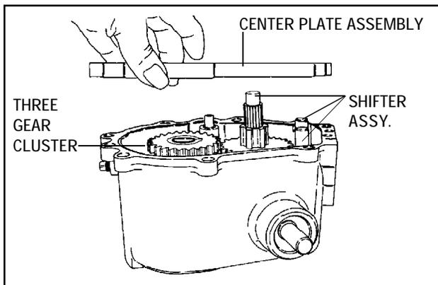
6. Remove temporary holding screws, if used and lift off center plate assembly. Discard gasket.
