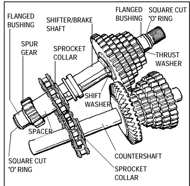
6. Angle the shifter/brake shaft and countershaft chain sprocket ends toward each other. Note the collar on the sprockets face the bevel gear. Remove chain.
