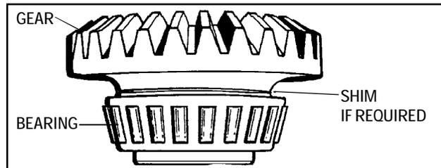
12. Press large shim and new large roller bearing on to gear using inner bearing race.
