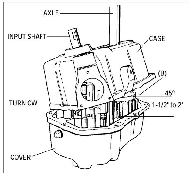
11. Position the gasket on the cover sealing surface, then install case over the differential shaft. Be sure the boss goes under gears and that edge of the case goes over the shaft rods in the opposite manner from which it was removed.
