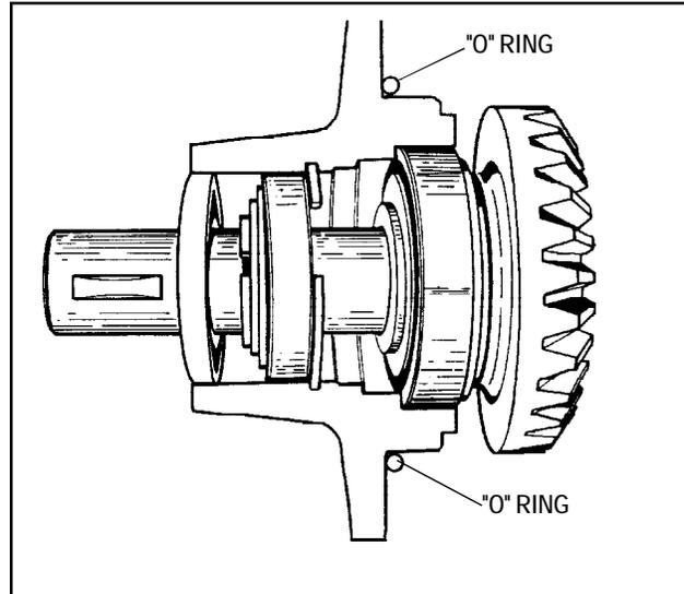
13. Place shaft into proper position in cage, push gear with bearing onto shaft.
