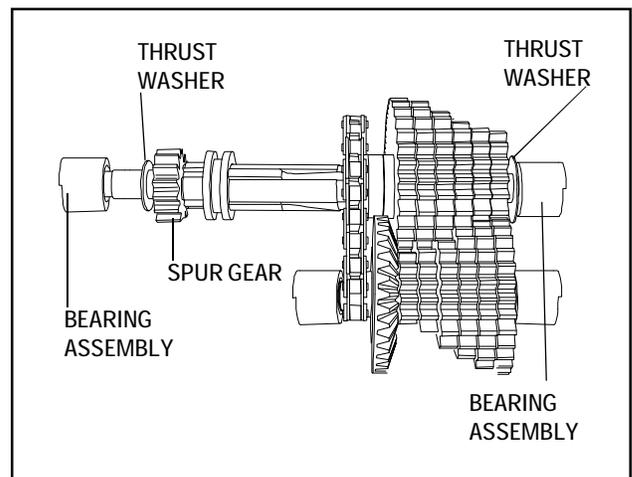
7. Place large thrust washer next to the last shifting gear (this may be a step washer on some models) then a sleeved needle bearing with "O" ring. Place the spur gear, small thrust washer and sleeved needle bearing with "O" rings on the opposite end of the shifter/brake shaft.
