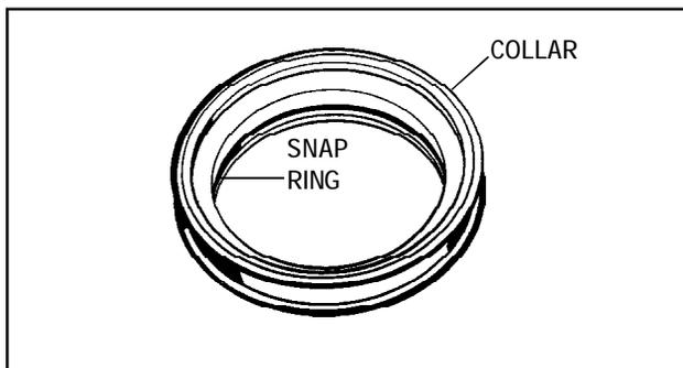
3. The collar has to be removed next. Place a jaw type puller around the collar and pull off. This will expose 3 steel balls equally spaced in holes around output shaft. There will be a snap ring in the inside of the collar. After the collar is pulled off discard snap ring.
