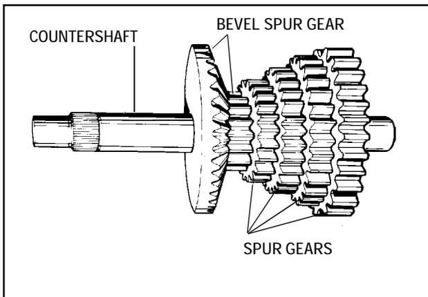
2. Remove bevel spur gear combination and spur gears from the countershaft; these gears are splined to the countershaft.
