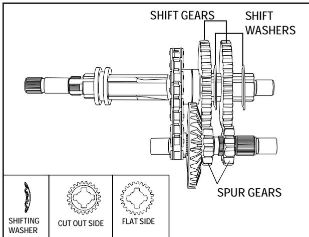
5. Build the gears on the countershaft and shifter/brake shaft alternately, meshing each gear with its mating gear on the other shaft. The first gear on the shifter/brake shaft would be the largest of the shifting gears. Place this gear next to the neutral spacer with the flat side of the gear next to the spacer. Place a shifting washer onto the shifter/brake shaft with the rounded edge towards the shifting keys. Continue this procedure until all the gears on both shafts have been added.
