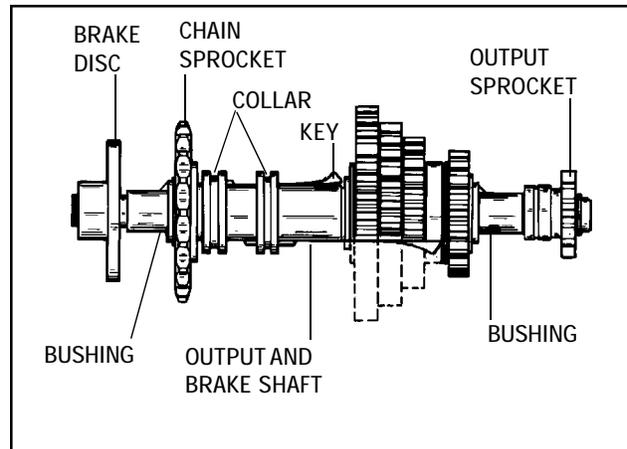
Correct assembly for 700 Model "H" shift pattern.
