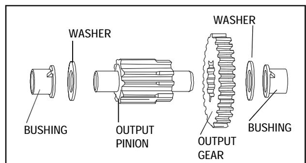
8. Place the output gear on the stepped end of the output pinion. Place the thrust washers on each end and then the bronze bushings. Install these 3 shaft assemblies back into the case. Make sure that the tabs of all the bushings are in their "V" notches in the case.
