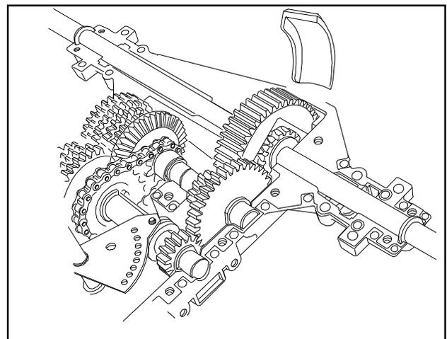
5. Remove the top bearing block on the bull gear of the differential. Remove the bull gear, bevel pinion gears with center shaft and the axles.
