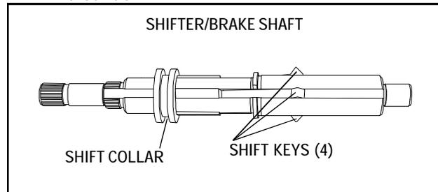
2. Grease all four keyways, insert keys into collar and keyways and slide onto the shifter/brake shaft.
