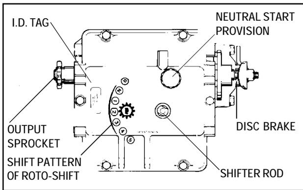
The two speed unit is not covered here but can be disassembled and reassembled using the same information for the 700 described in this section. Optional features include right or left hand output and disk brake, for either in-line or "H" pattern unit.
