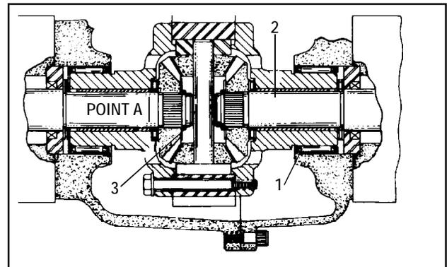
3. The 2000 series, three speed and the 2300 series, four speed differential. Examine the external bearing race on the differential carriers (1) for wear or pitting. Replace if evident. The differential carriers in this assembly have replaceable bushings (2). Replace if worn in
