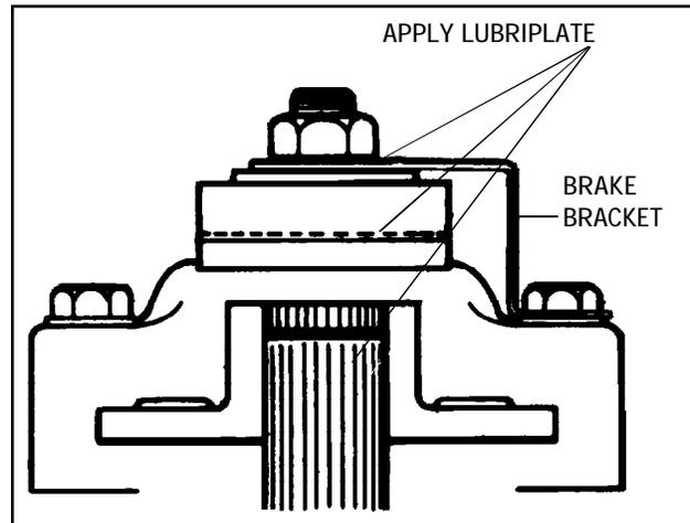
16. Prior to installing the brake assembly, apply a light film of lubriplate to the inside of lever portion which contact pins, also to outside of lever which contacts flat washer and between shaft O.D. and bore of brake disc. Brake pads and brake disc must be free of grease and oil. Install brake assembly.
