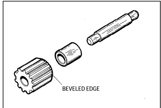
8. Remove reverse idler shaft, spacer and gear.
