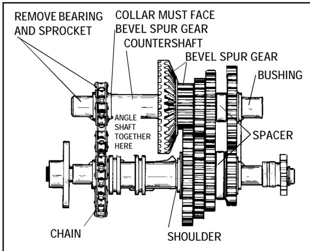
With collar on countershaft sprocket facing the bevel spur gear, install sprocket onto serration and install chain. Install all (4) thrust washers, **MUST** be positioned on the shifting gear of the output shaft.
