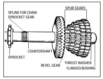
5. Install bevel gear and smallest to largest spur gears, thrust washer and bushing to the counter shaft. Install the sprocket.
