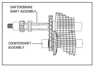
6. COUNTERSHAFT AND SHIFTER/BRAKE SHAFT
