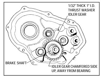
14. Remove the brake shaft.
