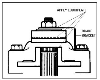
11. Apply a light film of lubriplate to the inside of lever portion which contacts pins, also to outside of lever which contacts flat washer and between shaft O.D. and bore of brake disc. Brake pads and brake disc must be free of grease and oil.
