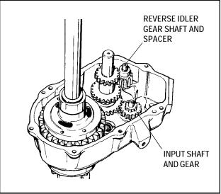
7. Remove the reverse idler shaft, spacer and gear.
