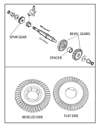
3. The large beveled shifting gears can be placed onto the shifter/brake shaft. The bevels on the gears face each other and are separated with a neutral spacer. Push shifting keys into the neutral spacer.
