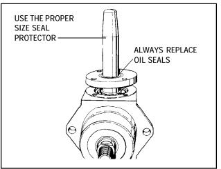
12. Install new oil seal, using seal sleeve No. 670293 and driver until seal is flush with housing.
