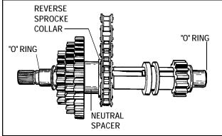
3. Place the reverse chain on the reverse sprockets. The collars of the reverse sprockets should be on the same side of the chain. Slide the larger sprocket onto the shifter/brake shaft with the collar away from the shifting keys and shoulder on the shifter/brake shaft. Slide the keys through the sprocket and install the neutral spacer over the ends of the shifting keys and pull them back until the sprocket touches the shoulder of the shaft.
