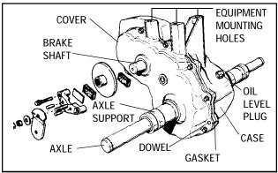
Axle supports, pressed from the inside out, must be removed with the case and cover, similar to the method used in the 1200 series transaxle.
