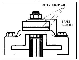
16. Prior to installing the brake assembly, apply a light film of lubriplate to the inside of lever portion which contact pins, also to outside of lever which contacts flat washer and between shaft O.D. and bore of brake disc. Brake pads and brake disc must be free of grease and oil. Install brake assembly.
