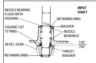
The input shaft can also be removed and inspected or serviced. Remove the snap ring on the bevel gear and pull the shaft through the case. The square cut "O" ring must be replaced if the shaft is removed.
