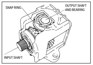
d. The top ball bearing in the blind end of the housing, is removed by either heating the housing on a hot plate or tapping the housing on the outside with a mallet.
