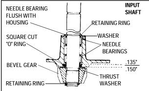
10. Remove retaining ring on bevel gear side from the input shaft, remove bevel gear and pull shaft through case. The square cut "O" ring must be replaced, if removed. Tool Part No. 670251 is used for removal and installation of needle bearings for the input shaft. The needle bearing on inboard side is installed .135/.150" below flush.
