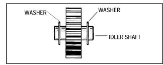
3. Place idler gear into case with washers on both sides along with output shaft at the same time.
