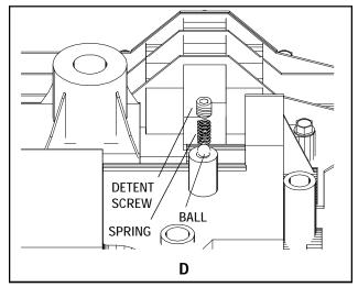
6. Remove the set screw, spring and index ball (See Illustration D).
