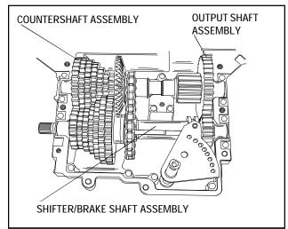
6. There are 3 shaft assemblies in this transaxle; the output shaft, the countershaft, and the shifter/brake shaft assembly. Remove these assemblies as complete as possible from the case.
