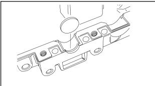
11. To seal the case and cover at the end of the shifter/brake shaft, a flat plug is placed there (end opposite the brake assembly). Clean the mating surfaces of case and cover; place a continuous thin bead of sealant all around the seam. Use Loctite Gasket Eliminator #515, Tecumseh part number 510334 or the Loctite Silicone RTV 598, Tecumseh part number 788093.
