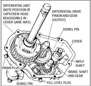
f. Before removing differential unit, note the position of the cap screw heads. Replace the unit in the same way to insure that axle lengths will be correct when installing axle supports.
