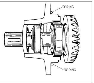
13. Place shaft into proper position in cage, push gear with bearing onto shaft.
