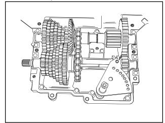
10. Install the shifter assembly and bearing strap, pack the transaxle with the remaining Bentonite grease (30 ounces total). Apply grease to top of shift fan.
