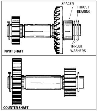
2. To remove components in the single speed, first remove the differential, thrust washers, drive gear, input shaft, countershaft, output gear and shaft.
