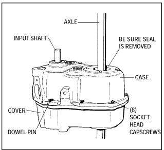
5. Tap dowel pins into the cover and remove the socket head capscrews.
