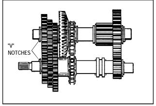
Remove gear and shaft assemblies from case half. NOTE: Before disassembly, observe how "V" notches on the flange bushings fit into recess "V" of case.
