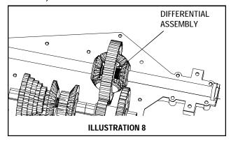
6. To reassemble the differential, first inspect the axle bevel gears for damage or wear. If it is necessary to replace a gear, the mating gears must also be replaced. The differential must be assembled outside of the case and placed into the case as an assembly (Illustration 8).
