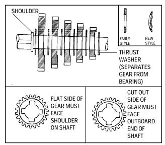
3. Install the thrust washers and shifting gears onto the shifter/brake shaft. The number of gears and/or spacers will be determined by the number of speeds in the transmission.
