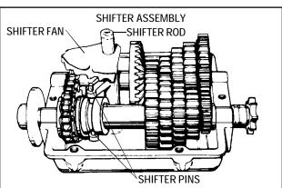
Install shifter assembly (shaft, pins and fan) 12 oz. Bentonite grease around gearing, and reinstall cover on case. Torque cap screws 90-110 in. lbs.
