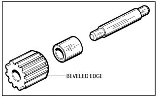
9. Install the reverse idler shaft, spacer and gear in to the cover. The beveled side of the idler gear should be down into the cover.
