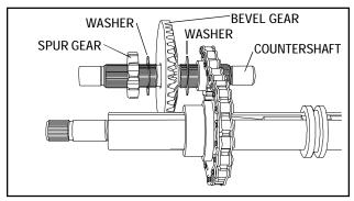
\*4. Insert the countershaft into the smaller reverse sprocket. Insert a thin thrust washer next to the sprocket (collar side) and then install the large bevel gear, with the bevel towards the reverse sprocket. Place another thin thrust washer on the back side of the bevel gear.
