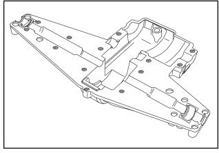
7. Remove the shifter/brake shaft assembly.
