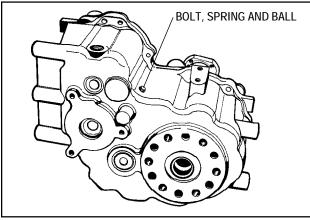
a. To remove the shifter rod and fork, remove the outside bolt, spring and ball. Remove high range gear then shifter gear cluster and fork assembly together.
