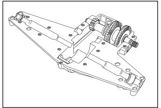
6. Remove the output shaft assembly.
