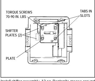
Install shifter assembly, 12 oz. Bentonite grease around gearing, and reinstall cover on case. Torque cap screws 90-110 in. lbs.
