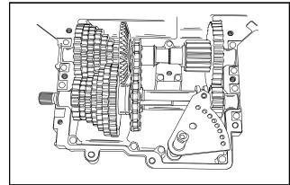
10. Install the shifter assembly and bearing strap, pack the transaxle with the remaining Bentonite grease (30 ounces total). Apply grease to top of shift fan.
