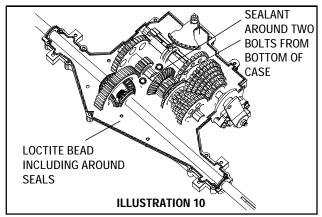
7. To seal the case and cover. Clean the mating surfaces and place a continuous thin bead (1/16") of Loctite 598 Silicone RTV (part # 788093) around the entire perimeter of the cover to prevent oil from leaking INCLUDING CASE AND COVER SEAL POCKETS. Caution must be used when locating this bead so that oil passages that lead to the axle shafts don't become blocked and prevent lubrication in these critical areas. Don't forget the two bottom bolts (Illustration 10).
