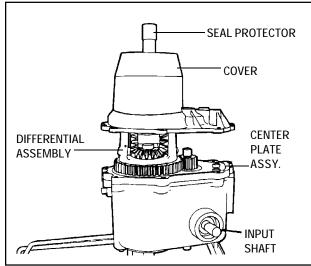
4. Use a seal protector on axle shaft and lift off transaxle cover assembly. Because this seal is a single lip type, it may be reused, if care is taken to see that it isn't cut or scratched. Discard gasket.
