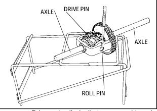
a. Drive out roll pin that secures drive pin with suitable driver.
