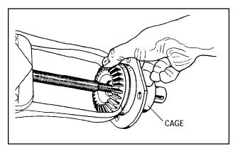
3. To disassemble the input cage assembly, first remove the nut and washer that holds the large keyed gear onto the shaft. With an outside puller, if necessary, remove gear. Roller bearings will be attached.
