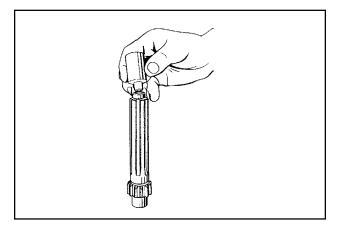
e. Use the authorized tool to install the new bearing. Needle bearings in shifter shafts should be installed .010'' below flush.
