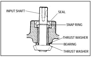
12. Remove input shaft oil seal to allow access to snap ring. Remove snap ring and input shaft will slide out. A removed seal must be replaced by a new seal.
