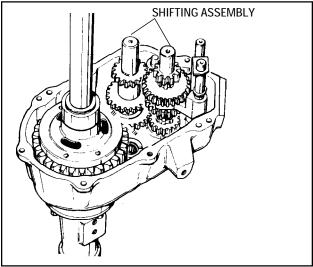
6. Remove the shifting assembly as one unit.
