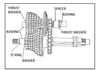
\*6. Place the spacer on the countershaft next to the reverse sprocket. Then place a thrust washer on each end of the countershaft and insert the bronze bushings.
