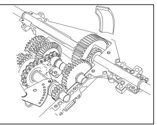
5. Remove the top bearing block on the bull gear of the differential. Remove the bull gear, bevel pinion gears with center shaft and the axles.
