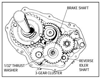
10. With the small gear of the three gear cluster toward the spacer, install the three gear cluster and other 1/32" thick by 7/8" I.D. thrust washer on the brake shaft.
