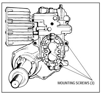
a. To separate the units, block the assembly to prevent falling, then remove the three hydrostatic mounting screws. Lift either unit from the other. If any binding occurs, remember that the drive shafts are held in common rotation by a splined coupling and the coupling may have a slight bind on the driveshafts.
