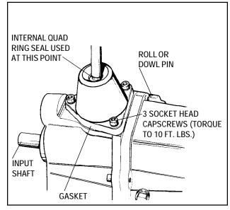
16. Install shift lever housing and new gasket.
