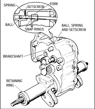
2. To remove the shifter rod and fork, the set screw, spring and ball should be removed at the outside of the case.
