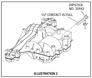
Insert dipstick Part Number 35942. Insert the gauge at a 45° angle. Check for approximately 1/2 inch of oil when inserted. This is 16 ounces of EP90 gear oil (Illustration 2).
