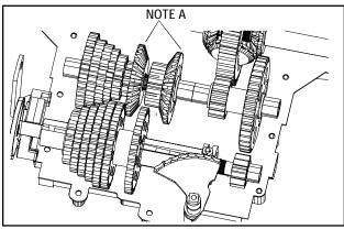
5. There are 3 shaft assemblies in this transaxle. The countershaft, shifter/brake shaft and output shaft. Remove shifter fork assembly and then remove these assemblies from the case.
