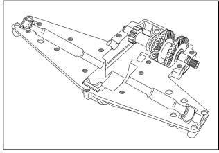
4. Place the shifter/brake shaft assembly in the case.
