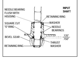
The input shaft can also be removed and inspected or serviced. Remove the snap ring on the bevel gear and pull the shaft through the case. The square cut "O" ring must be replaced if the shaft is removed.
