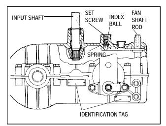
12. Install index ball, spring and setscrew in that order into cover, and slowly tighten the screw 1 turn below flush. If unit contained a neutral start switch install. Check for binding by turning input shaft.
