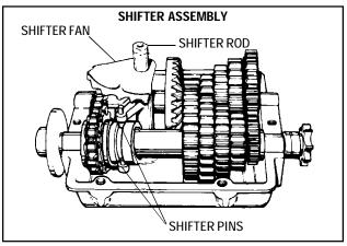
3. Remove cover. Remove shifter assembly (includes shafts, pins and fan from transmission by lifting shaft out of case.
