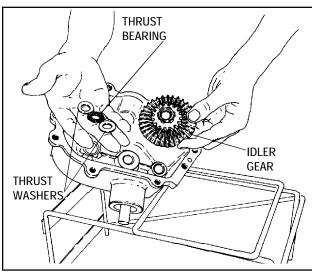
b. Set case assembly open side up. Insert the idler gear assembly, thrust washers and bearing. Note sequence of washer and bearings from case, thick washer, thrust bearing thin washer, idler gear.
