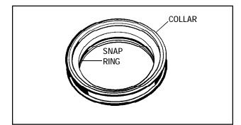
3. The collar has to be removed next. Place a jaw type puller around the collar and pull off. This will expose 3 steel balls equally spaced in holes around output shaft. There will be a snap ring in the inside of the collar. After the collar is pulled off discard snap ring.
