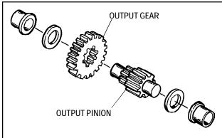
5. Place the output gear onto the output pinion. Install the thrust washers and bushings.
