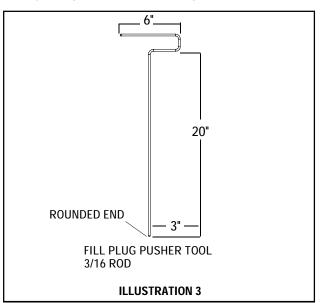
A. When the plug is accessible from the battery box area, make an installation tool from 3/ 16 cold rolled steel rod as shown (Illustration 3).
