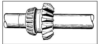
2. When pressing roller bearings into place with press, make sure inner bearing race is used.
