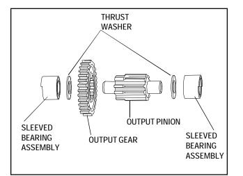
8. Place the output gear on the stepped end of the output pinion. Place thrust washers on each end and then the large sleeved needle bearings. Install the three shaft assemblies into the case.
