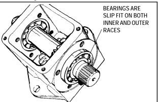
4. Press input shaft ball bearings out of the housing with fingers. If they stick, tap lightly using a drift punch around the outer race.
