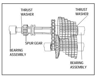
7. Place large thrust washer next to the last shifting gear (this may be a step washer on some models) then a sleeved needle bearing with "O" ring. Place the spur gear, small thrust washer and sleeved needle bearing with "O" rings on the opposite end of the shifter/brake shaft.
