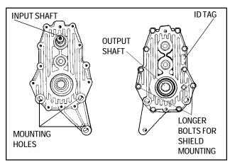
The Model 2800 series transmission is the first of its kind produced by Peerless. It's known as a P.T.O. (Power Take Off) unit. This unit mounts on the back side of the Model 2600 series transaxle. Some O.E.M.'s are using this unit to run auxiliary attachments such as large tillers, mower decks, or any attachments that need power to make them operate.
