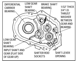
1. Install input shaft in case. Use a soft mallet to seat shaft and gear completely. Often, binding in the assembled unit can be traced to a partially installed input shaft.
