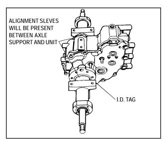
b. To remove axle out of support, tap lightly with a mallet from inside out. A pressed on sealed bearing will be on the end of axle.
