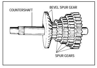
5. Install bevel spur gear and smallest to largest spur gears to the splined end of the counter shaft.
