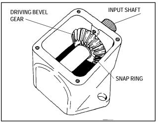
3. Remove four screws and the cover and seal assembly.
