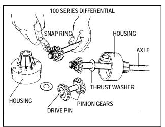
d. Remove snap ring, bevel gear and thrust washer. Slide axle from differential carrier housing.
