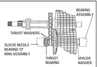
6. In the model pictured, a thrust washer, thrust bearing, thrust washer and sleeved needle bearing with "O" ring are placed on the countershaft next to the reverse sprocket. Place a spacer washer and sleeved needle bearing with "O" ring next to largest spur gear. The sleeved needle bearing installation will have the step facing outward and the wider portion of the bearing sleeve toward the cover. This will be true for all future sleeve bearing installations.
