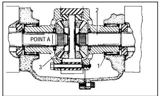
The 2000 series, three speed and the 2300 series, four speed differential. Examine the external bearing race on the differential carriers (1) for wear or pitting. Replace if evident. The differential carriers in this assembly have replaceable bushings (2). Replace if worn in
