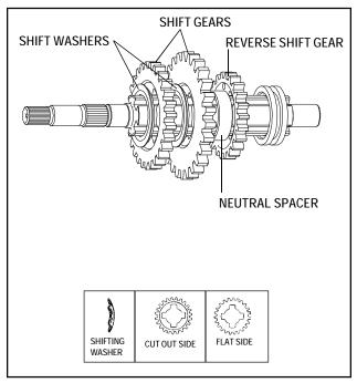
**NOTE:** As all the gears are placed back into the assembly, each should be packed with Bentonite grease.
