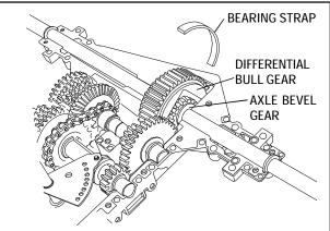
5. Remove the bearing strap on the bull gear of the differential. Some models do not use a bearing strap. Remove the bull gear, bevel pinion gears with center shaft and the axles. Grasp the axle bevel gears between your thumb and fingers, hold together while lifting differential from case.
