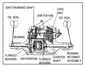
Remove gear and shaft assemblies from case half by lifting the two shafts out of the bearing supports taking care not to disturb drive chain relationship with hubs on sprockets.
