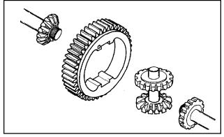
**NOTE:** The differential must be assembled out of the case and then placed in the case. Apply Bentonite grease to axle contact areas of case.
