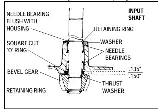
The input shaft can also be removed and inspected or serviced. Remove the snap ring on the bevel gear and pull the shaft through the case. The square cut "O" ring must be replaced if the shaft is removed.
