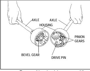
c. Remove drive pin, pinion gears and thrust washers as a unit.
