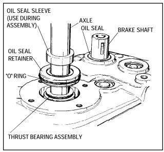
15. Install new "O" rings on seal retainers and position axle supports to case and cover. Be sure mounting pads face in the same direction as when removed. Install capscrews and torque to 13 ft. lbs.
