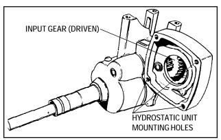
After removing the hydrostatic unit, inspect the 2. surfaces and the gears from outside unit.
