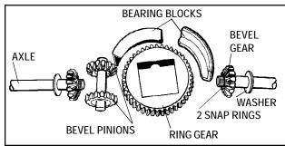
When assembling this unit, make sure all parts are there first, because the unit is put together in your hands and placed in the case at the same time.
