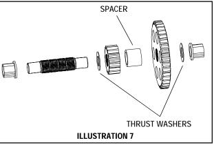
The output shaft is completely splined and consists of a bronze bushing, thrust washer, a large output gear, spacer, small output gear, thrust washer and bronze bushing. (Illustration 7)
