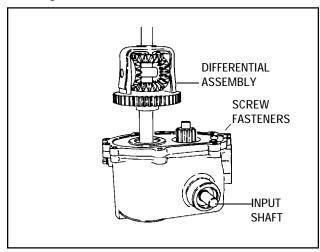
To remove differential assembly, it may be necessary to replace two or three screws to hold center plate assembly down. Pull assembly straight up. If tight, tap on lower axle with soft mallet. CAUTION: DO NOT USE STEEL HAMMER. Refer to the chapter on differential assembly service. Remove gear on top of shifter shaft.
