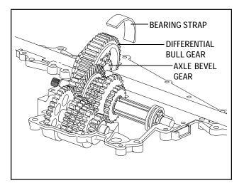
6. Remove the bearing strap on the bull gear of the differential. Remove the bull gear, bevel pinion gears with center shaft and the axles. Grasp the axle bevel gears between your thumb and fingers, hold together while lifting differential from case.
