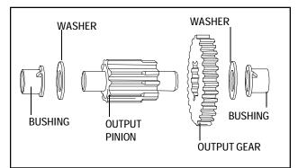
8. Place the output gear on the stepped end of the output pinion. Place the thrust washers on each end and then the bronze bushings. Install these 3 shaft assemblies back into the case. Make sure that the tabs of all the bushings are in their "V" notches in the case.
