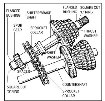
6. Angle the shifter/brake shaft and countershaft chain sprocket ends toward each other. Note the collar on the sprockets face the bevel gear. Remove chain.
