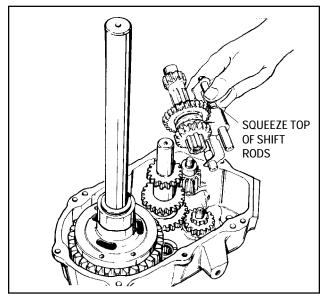
5. Install the shifter assembly as a unit into the case. When installed correctly, the neutral square formed by the shifting forks should appear through the case opening for attaching the shift housing. Both shift gears should be out of mesh.
