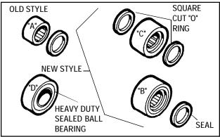
Remove differential from case. Remove seals (2), needle bearings or ball bearings (2), flanged bushings (2) and thrust washer.
