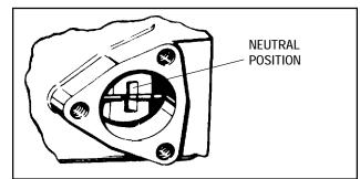
Clean the outside surface of the transaxle, away from the area where disassembly will take place. Position shift lever in neutral position to help disassembly. Remove screws (3) holding shift lever. Remove all keys from keyways, remove all burrs and dirt from shafts. On hardened shafts, use a stone to remove burrs. All seals should be replaced whenever a shaft is pulled through a seal. Always use a new gasket whenever the gasket surfaces have been separated.
