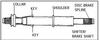
Grease the keyways and slide keys and collar on output and brakeshaft. Thick side of collar MUST face shoulder on shaft. Service replacement shifter/brake shafts will come with 4 keyways in the shaft instead of 2.
