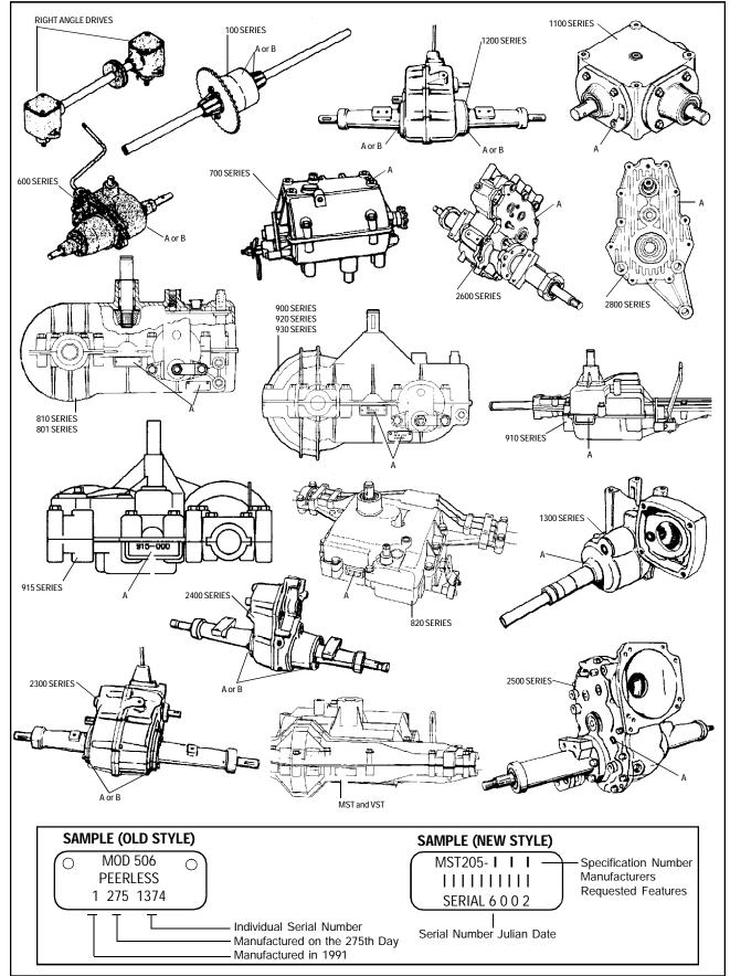
Early Models were not identified with a model number on the unit. THE MODEL NUMBER WILL BE FOUND ON: A. Metal tag or decal attached to unit as illustrated. B. Stamped on unit as illustrated.
