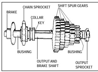
4. When correctly assembled the output shaft should appear as shown.
