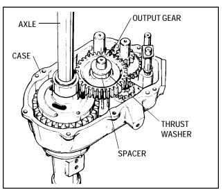
5. Lift the cover off from the case. Discard gasket. Remove output gear and shaft.
