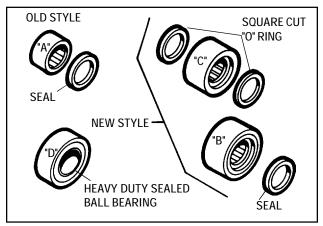
The 800 Series has used 4 styles of bearings on the axles. The earliest style "A" was a smaller loose cage needle bearing and must have the seal to the outside of that bearing. Style "B" must have the seal to the out side of the bearing. When bearing style "C" is used, a square cut "O" ring must be used on each side of the bearing. Bearing style "D" is a sealed ball bearing used in H.D. application. Styles "B", "C" and "D" are inter changeable. All needle bearings must be repacked with grease.
