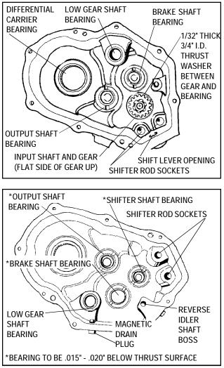
15. Remove input shaft from case by tapping with a non-metallic hammer.
