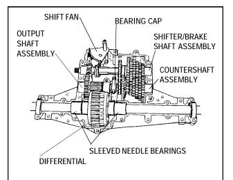
**NOTE:** Remove grease from the unit as parts are removed. Remove the shift fan prior to removal of the gear shaft assemblies from the case. It will be difficult to keep parts from falling off the assemblies, note position of parts before removal.
