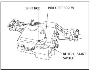
11. Guide cover over shift rod and position onto case. Torque cover screws 180-216 inch pounds. Replace index ball, spring and set screw and turn set screw one (1) turn below flush. Install the neutral start sensing switch if applicable. Check for binding by turning input shaft.
