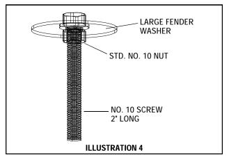
B. If working from the bottom or side, use a No. 10 screw approximately 2 inches long with full threads. Then find a large fender washer and nut for the screw. The washer will give your fingers a large surface area to push down on for re-installation of the plug (Illustration 4).
