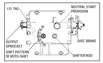
The two speed unit is not covered here but can be disassembled and reassembled using the same information for the 700 described in this section. Optional features include right or left hand output and disk brake, for either in-line or "H" pattern unit.
