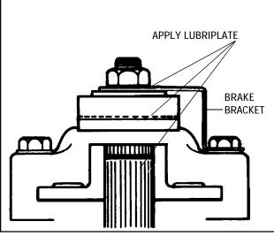
13. Prior to installing the brake assembly, apply a light film of lubriplate to the inside of lever portion which contact pins, also to outside of lever which contacts flat washer and between shaft O.D. and bore of brake disc. Brake pads and brake disc must be free of grease and oil. Install brake assembly.
