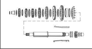
As these assemblies are taken apart, lay the parts out in a systematic order. This will help to make reassembly easier and inspection of all parts possible. Clean each part of grease as the parts are laid out.
