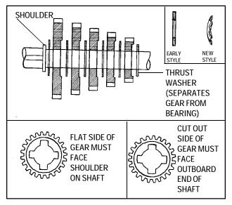
Install the thrust washers and shifting gears onto the shifter/brake shaft. The number of gears and/or spacer will be determined by the number of speeds in the transmission.
