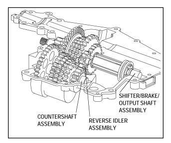
7. There are 2 shaft assemblies in this transaxle; the countershaft and the shifter/brake/output shaft assembly. Remove these assemblies as complete as possible from the case.
