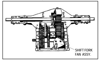
**NOTE:** Remove grease from the unit as parts are removed. Prior to removal of gear shaft assemblies from the case, the shifter fan may be removed. It will be difficult to keep parts from falling off the assemblies. Note position of parts before removal.
