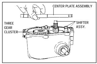
6. Remove temporary holding screws, if used and lift off center plate assembly. Discard gasket.
