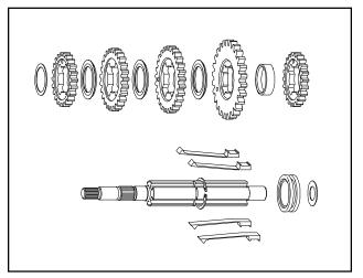
8. As these assemblies are taken apart, lay the parts out in a systematic order. This will help to make reassembly easier and inspection of all parts possible. Clean grease from each part as the parts are laid out. To remove keys from the shifter/brake/output shaft you must remove the large snap ring from its groove. Be careful not to stretch or twist snap ring, it is not necessary to remove snap ring from shaft.
