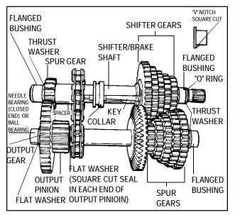
Install the output and pinion gears, the flat washer, square cut rings, needle bearing (closed end), and spacer on one end and thrust washer and flanged bushing on the other end. Note that the "V" notch on the bushing fits into recess "V" in case.
