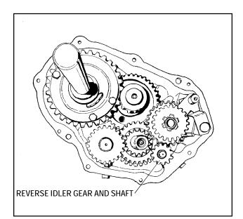
8. Remove the reverse idler gear, spacer and shaft from boss in cover. Note that the spacer goes between the gear and the cover, and that the gear bevels go down. Excessive wear on teeth bevels indicates improper shifting technique.
