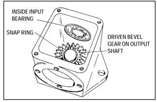
7. The ball bearing that supports the inner end of the in put shaft is removed by holding the housing in the hand and tapping the housing sharply on the outside with a soft mallet behind the bearing. It may at times be necessary to heat the housing to remove this bearing.
