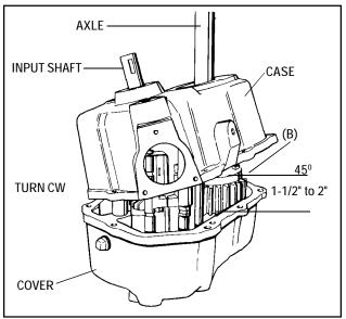
11. Position the gasket on the cover sealing surface, then install case over the differential shaft. Be sure the boss goes under gears and that edge of the case goes over the shaft rods in the opposite manner from which it was removed. 12. Once in position, if case hangs 1/2 to 1'' high, turn the input shaft to get gears to mesh. The case should drop about 1/4'' from closing.
