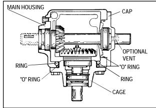
The 1100 series angle drive is a heavy duty gear box used with larger equipment with a larger H.P. rating up to 20 H.P. This unit is of cast iron construction for strength and tapper roller bearing for longer life. This unit can be either right angle drive with right or left handed rotation, or a "T" drive. Disassembly and reassembly are the same.
