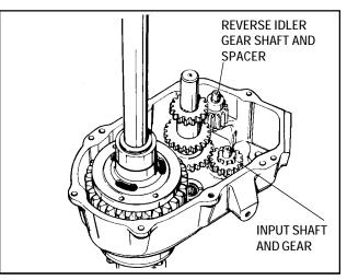
4. Position the reverse idler shaft in the unit, then install gear and spacer.
