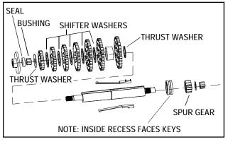
7. To disassemble the shifter/brake shaft, start on the spur gear side. Remove the oil seal, the bronze bushing and thrust washer. Remove all of the shifter spur gears (or spacers if used) and shift washers. Remove the neutral collar, reverse gear and thrust washer. On the output side of the shifter/brake shaft remove the bronze bushing, thrust washer, and output spur gear.
