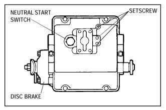
If installed, (optional equipment), remove neutral start switch.
