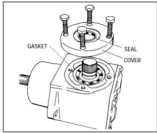
Leaking lubricant: Correct lubricant leakage by replacing the seals at the input and output shaft as described above.
