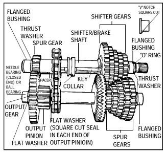
**NOTE:** Before disassembly, observe how "V" notches on the flanged bushings fit into recess "V" of case.
