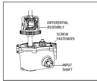
g. Place new gasket on center plate and install differential assembly, longer axle in down position. Be sure gear on shifter shaft is on shaft.
