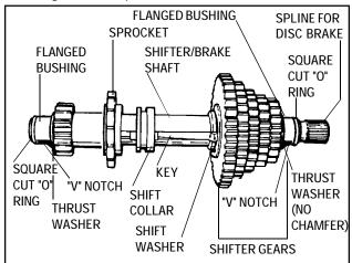
8. Remove the square cut seals (2) and flanged bushings (2), thrust washers (2) on shaft ends, spur gear, spacer, sprocket, shift collar with keys, thrust washers and shifter gears.
