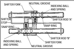
4 Stop, 4-Speed Transaxle Shifter Rod & Fork Assy.
