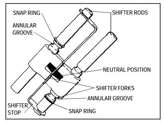
When the shifter forks are properly assembled to the shifter rods and positioned in neutral, the ends of the notches in the shifter forks are in alignment.
