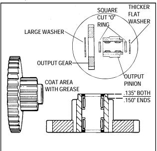
For correct positioning of the needle bearings use removal and installation Tool Part No. 670252. Fill the area between the needle bearings with grease before installing on the countershaft.
