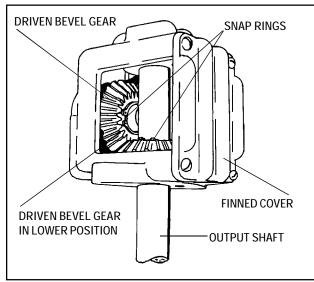
a. If the driven bevel gear is on the bottom, remove the snap ring on the output shaft and pull out the output shaft.
