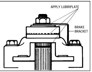
12. Prior to installing the brake assembly, apply a light film of lubriplate to the inside of lever portion which contact pins, also to outside of lever which contacts flat washer and between shaft O.D. and bore of brake disc. Brake pads and brake disc must be free of grease and oil. Install brake assembly.
