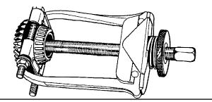
\*4. Remove bearing from gear by using a bearing splitter and puller.
