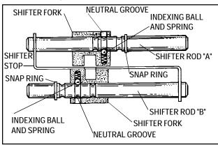
1. Assemble the shifter forks to the shifter rods. The shifter forks are interchangeable.
