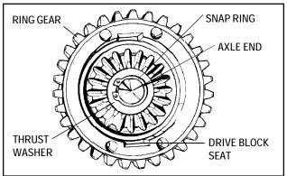
3. Remove the snap ring and the thrust washer, if used. Separate the bevel gear and the differential carrier from the axle.
