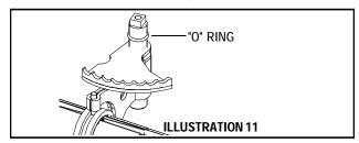
Before placing the cover on the case, place the shift rod and fork pins into the shift collar and shaft into the boss in the case. Inspect the shaft on the rod and fork for rust and burrs. (Illustration 11)
