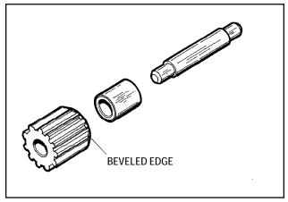
e. Install reverse idler. Make sure beveled edge is up. Spacer on top of gear.
