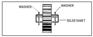
9. Remove the idler shaft and two washers.
