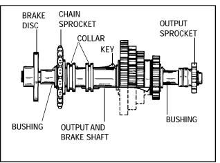
Correct assembly for 700 Model "H" shift pattern.
