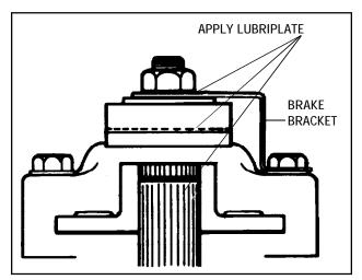
Apply a light film of lubriplate to the inside of lever portion which contacts pins, also to outside of lever which contacts flat washer and between shaft O.D. and bore of brake disc. Brake pads and brake disc must be free of grease and oil.
