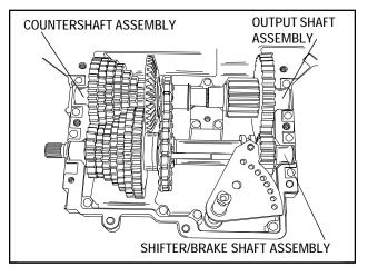
There are 3 shaft assemblies in this transaxle; the output shaft, the countershaft, and the shifter/brake shaft assembly. Remove these assemblies as complete as possible from the case.
