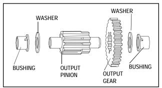
8. Place the output gear on the stepped end of the output pinion. Place the thrust washers on each end and then the bronze bushings. Install these 3 shaft assemblies back into the case. Make sure that the tabs of all the bushings are in their "V" notches in the case.
