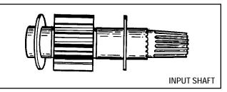
7. Remove the input shaft and two washers. The input shaft and gear are one piece.
