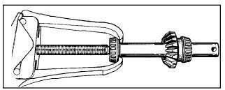
8. To disassemble the output shaft assembly<sup>\*</sup>, first remove the bearing that is located under cap on shaft, by using an outside puller.
