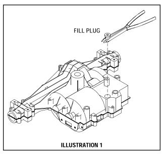
4. With a needle nose pliers or needle nose vise grip, work under the lip of the plug, rocking from side to side until plug is removed (Illustration 1).
