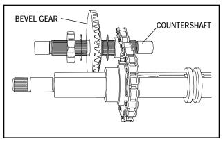
\*4. Insert the countershaft into the smaller reverse sprocket. Insert a thin thrust washer next to the sprocket (collar side) and then install the large bevel gear, with the bevel towards the reverse sprocket. Place another thin thrust washer on the back side of the bevel gear.
