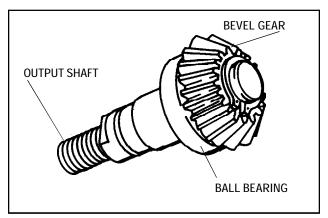
6. Remove the input shaft from the ball bearing, with an arbor press. Always support the inner race when removing and replacing the input shaft into the ball bearing. Use tool 670293 to support the inner ball bearing race.
