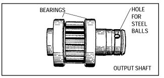
8. Remove output shaft. Output shaft bearings can be removed by using a bearing splitter and puller.
