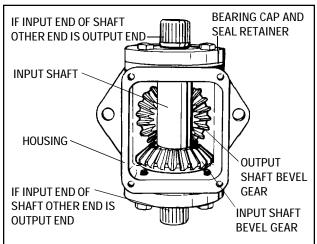
3. Remove capscrews and both retainer cap and seal assemblies. Separate and discard oil seals and gaskets.
