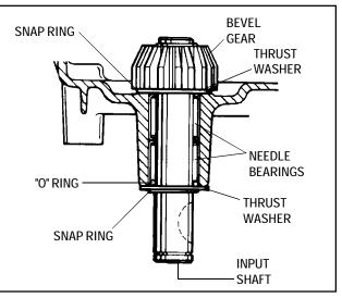
Input shaft removal for 700 series in-line transmission.
