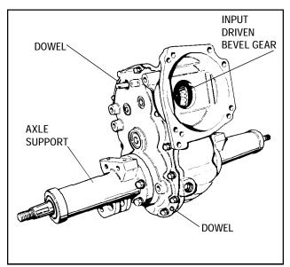
a. Remove the axle supports. If supports are different or if there is a chance for confused reassembly, scribe alignment marks.
