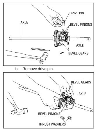
c. Thrust washers must be removed before attempting to remove the pinions. Remove bevel pinions simultaneously by rotating the gears in opposite directions; gears will move out of position.
