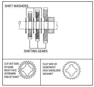
5. Place the largest of the shifting gears with the flat side of the gear next to the neutral spacer. Then place a shifting washer with the chamfer on the inside diameter of the washer next to the gear. The chamfer or rounded side must face towards the shifting keys.
