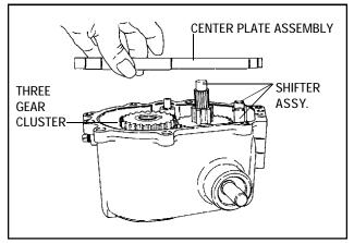
f. Place new gasket on case and install center plate.
