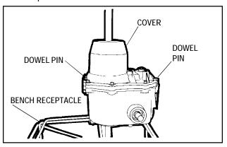
3. Remove the socket head cap screws holding the case and cover together. Drive out the dowel pins used for alignment of the case and cover.
