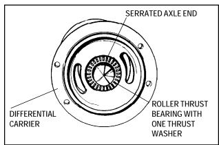
f. When assembling thrust bearings, always place a hardened thrust washer on each side of the caged thrust rollers. Never use the caged thrust rollers without the thrust washers.
