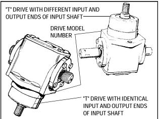
2. To disassemble "T" Drive, remove self-tapping screws and housing cover and clean grease from internal area. Note and mark near the casting gasket surface on the side where the beveled in put gear is located. To switch the "T" 180° will result in output shaft opposite rotation.
