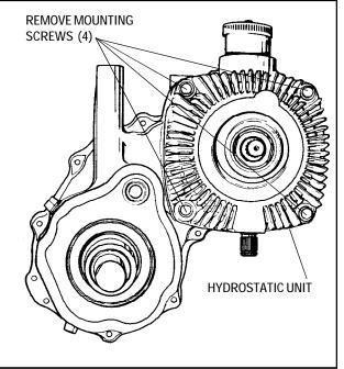
To separate the hydrostatic unit from the 1300, 1. support both parts, then remove the four mounting screws, and separate the parts. Drain oil from the 1300 unit. Any hydrostatic repair must be done through the equipment brand dealer.
