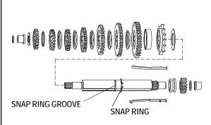
7. As these assemblies are taken apart, lay the parts out in a systematic order. This will help to make reassembly easier and inspection of all parts possible. Clean each part of grease as the parts are laid out. To remove keys from the shifter/brake shaft you must first remove the large snap ring from the snap ring groove. Be careful not to stretch or twist snap ring, it is not necessary to remove snap ring from shaft.
