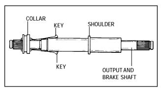
2. Install collar and keys on output shaft. Thick side of collar MUST face shoulder on shaft.
