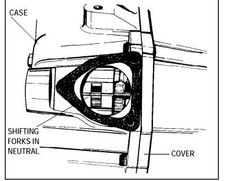
1. Position the shifter forks in neutral before disassembly.
