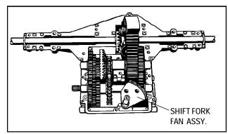
13. Install shifter assembly and pack 26 oz. Bentonite grease around bearings, gearing, and top of shift fan then reinstall cover on case. Torgue cap screws 90-100 inch pounds.
