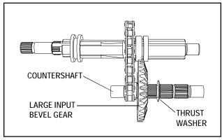
Insert the countershaft into the smaller reverse sprocket. Then install the large bevel gear, with the bevel facing away from the reverse sprocket. Place thin thrust washer on the countershaft next to the bevel gear.
