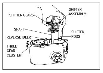
7. Remove complete shifter assembly by grasping shifting gears, shaft and both shifter rods as a unit.
