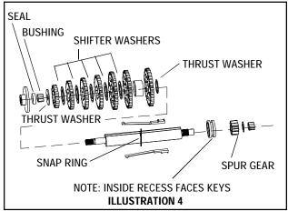
3. Place the plain large thrust washer over the key tips on the spur gear side of the shaft next to the snap ring. The sequence that follows is reverse gear then the neutral collar and 1st thru the amount of gears the unit is equipped with up to 6 gears (largest to smallest). Between each gear place a shift washer. Bevel facing keys. (Illustration 4)
