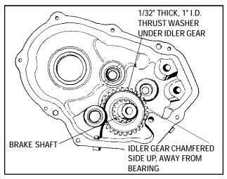
2. Center one 1/32'' thick by 1'' I.D. thrust washer on the cover brake shaft needle bearing, then in stall the brake shaft and gear, (chamfer side away from cover).
