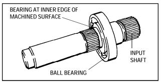
2. If the unit is built with the bevel gear on the input shaft toward the cover, remove the snap ring on the input shaft from the groove.
