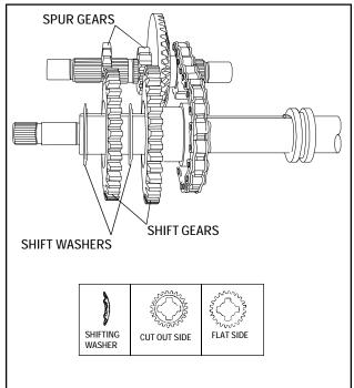
5. Build the gears on the countershaft and shifter/ brake shaft alternately, meshing each gear with its mating gear on the other shaft. The first gear on the shifter/brake shaft would be the largest of the shifting gears. Place this gear next to the neutral spacer with the flat side of the gear next to the spacer.
