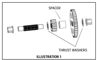
9. To disassemble the output shaft, remove the bushing, thrust washer, large output spur gear, spacer, small output spur gear, thrust washer, and bushing. (Illustration 1)
