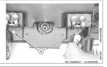
8. Loosen belt adjuster (A), using a screwdriver or bar to keep the adjuster from cocking as it is loosened.
