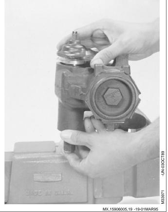
10. Remove preload adjuster and shim, if equipped, from side cover.
