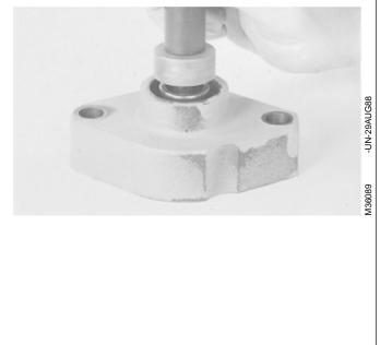
4. Install new O-ring (B). Apply petroleum jelly to seal and housing to hold O-ring in its groove.
