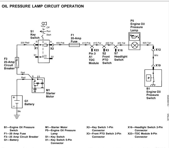
The purpose of the oil pressure lamp circuit is to warn the operator when engine oil pressure is too low for safe operation of the engine.
