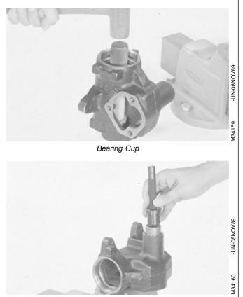
Needle Bearing MX,15906005,32 -19-01MAR95 3. Install new pitman shaft and worm shaft seals into gearbox housing using drivers from JDG457 Steering Gear Service Set.
