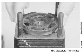
16. Remove and inspect hex drive assembly. Check sides and slot for wear, grooves, or scoring. Pin (A) should be tight and show no wear or damage.
