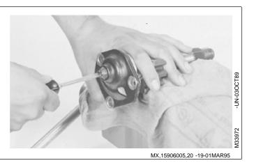
11. Remove worm bearing adjuster lock nut using a punch and hammer.
