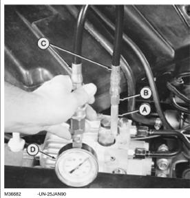
A—JT03339 Connector B—JT03107 Adapter C—JT03017 Hose D—JT03345 Gauge 20,000 kPa (3,000 psi) MX,159027020,18-19-24APR95
