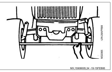
4. Loosen jam nuts and adjust tie rod to lengthen or shorten distance.
