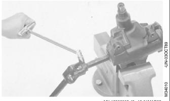
32. Install steering shaft onto worm shaft as shown. Tighten cap screws to 24 N·m (212 lb-in.).
