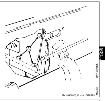
18. Remove steering gearbox and shaft as an assembly, from bottom of machine.
