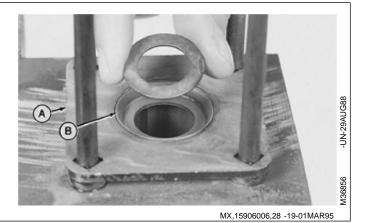
IMPORTANT: Hold steering tube in a soft-jaw vice. Be careful not to crush steering tube.
