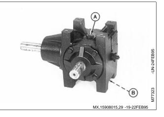
2. Remove four cap screws (A).
