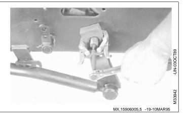
10. Remove cotter pin (A) and washer (B) to disconnect brake llinkage on left side of machine frame.
