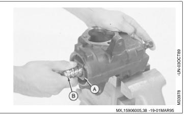
14. Install new bearing cup in worm bearing adjuster, if removed, using a driver set.
