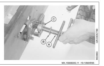
17. Remove three cap screws (A) from gearbox mounting plate.
