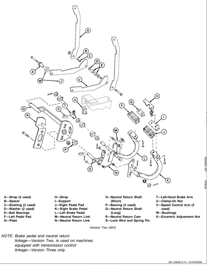
Brakes/Brake Pedal(s) and Neutral Return Linkage
