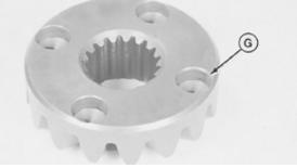
A—Pinion Gear (2 used) B—Pinion Block (2 used) C—Bevel Gear (2 used) D—Cross Shaft E—Ring Gear F—Carrier (2 used) G—Bevel Gear with Holes
