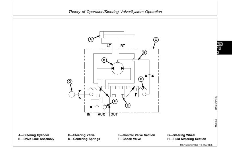
Theory of Operation/Steering Valve/System Operation
