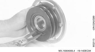
5. Remove hub and bearing from armature using a press and a 1-11/16 in. driver disk. Make sure assembly is supported on pulley, NOT on armature plate.
