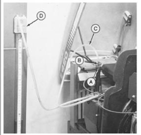
A—AHT8741-F66 Plug B—JT05703 Double Barb Fitting C—JT05699 Clear Line D—JT05698 U-Tube Manometer
