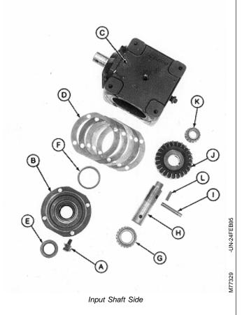
A—Cap Screw and Lock Plate (4 used) B—Cap C—Gear Case D—Shims (as required) E—Seal F—Bearing Cup G—Bearing Cone H—Input Shaft I—Spring Pin J—Bevel Gear K—Bearing Cone L—Key
