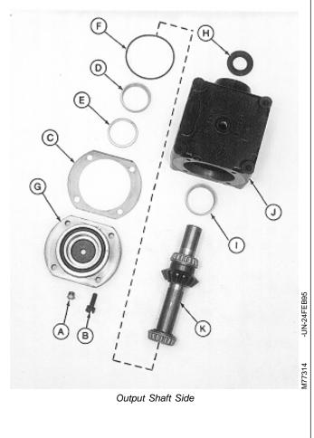
A—Vent Plug B—Cap Screw (4 used) C—Shim (as required) D—Bearing Cup E—Crush Ring F—O-Ring G—Retainer H—Seal I—Bearing Cup J—Gear Case K—Output Shaft Assembly
