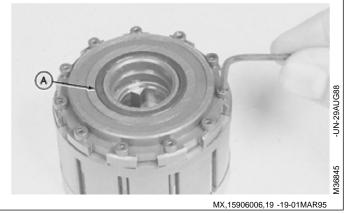
IMPORTANT: Handle commutator ring with care; it is easily broken.
