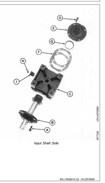
22. Remove input shaft assembly from cap (A).
