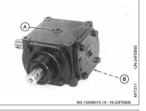
2. Remove four cap screws (A) and input shaft assembly.
