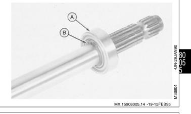
6. Inspect caged needle bearing (A) for wear or damage. Replace if necessary.
