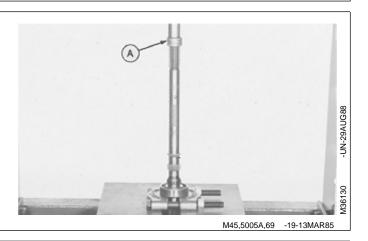
NOTE: Tape over splines to protect seals from possible damage when installing shafts, remove tape after installation.
