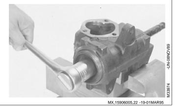
IMPORTANT: Do not allow worm shaft to turn to the end of its travel or damage can occur to the ends of the ball guides.
