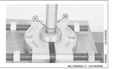
4. Support pivot pin on a press. Install PTO shaft assembly into pivot pin.
