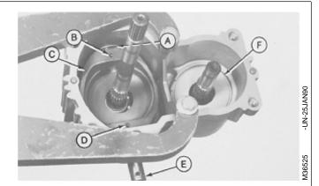
A—Trunnion Shaft **B—Spring Pin** C—Pump Swashplate D-Spring Pin (2 used) E-Control Shaft F-Motor Housing
