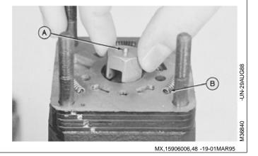
42. Apply petroleum jelly on new seal rings (A). Install seal rings on valve ring.
