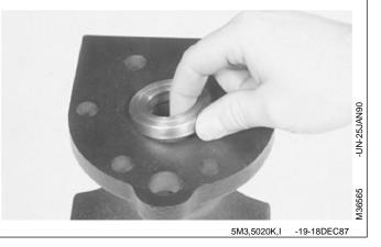
18. Remove seal from differential using a 2-jaw puller and a slide hammer.
