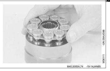
4. Install pump and motor cylinder blocks.
