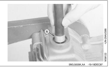
IMPORTANT: Be sure to hold shaft and bearing when removing from housing.
