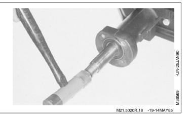
9. Clean the threads of all four brake plate cap screws and threaded axle housing using Clean and Cure Primer.
