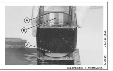
IMPORTANT: Do not clamp metering assembly in a vise.
