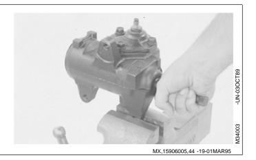
NOTE: Due to tolerances, some 11/16 in. sockets require a wrapping of card stock around the serrations on end of worm shaft.
