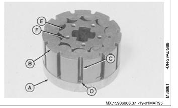
17. Apply multipurpose grease on spacer.
