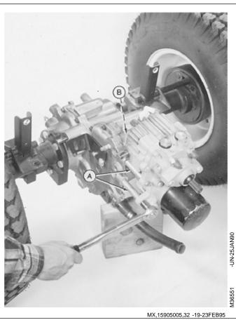
4. Position differential assembly under tractor.
