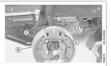
A—Cap Screw (4 used) B—Brake Plate Assembly C—Brake Support D—Lock Plate
