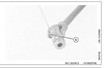
3. Remove cross and bearing assembly using soft metal rod. Push bearing down until it can be removed.
