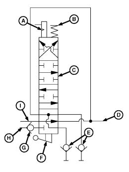
A—Detent B—Centering Spring C—Control Valve Spool D—Return Oil to Transmission E—Hydraulic Outlets F—Actuator G—Check Valve
