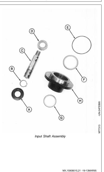
12. Remove vent plug (A) from retainer (G).
