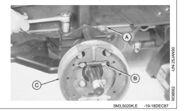
12. Remove axle shaft assembly using a bearing puller (A), H-Bar (B), and slide hammer (C).
