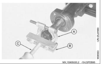
13. Inspect bearing (A), replace if necessary.
