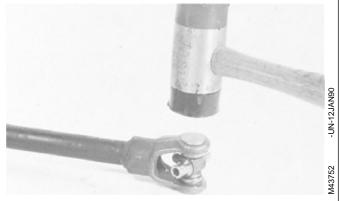
MX,15905025,8 -19-20MAR95 316, 318 & 420 Lawn and Garden Tractors 2. Install cross in splined yoke with grease fitting toward splined yoke (A).
