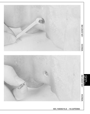
15. Remove and inspect intermediate shaft assembly; if equipped with two-speed differential, remove shift rod assembly with intermediate shaft.
