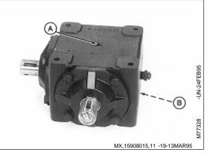
3. Remove four cap screws and lock plates (A).
