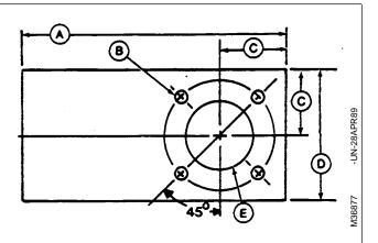
\*Four diameter holes equally spaced on a 83 mm (3-1/4 in.) diameter circle.
