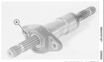
MX,15908005,12 -19-15FEB95 316, 318 & 420 Lawn and Garden Tractors 2. Push PTO shaft (A) and bearing (B) from pivot pin using a press.
