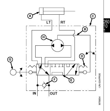
A—Steering Cylinder B—Drive Link Assembly
