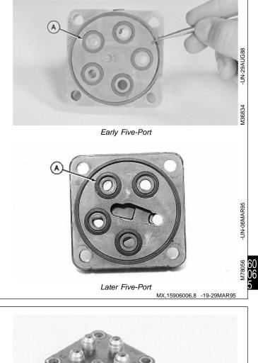
9. Four-port and early five-port; Remove plug (A), O-ring (B) and check ball (C).
