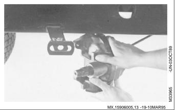
20. Inspect steering shaft bushings for wear or damage. Replace if necessary.
