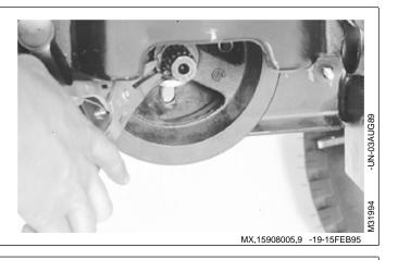
12. Remove two pivot pin retaining nuts (A).
