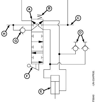
A—Control Valve Spool B—Centering Spring C—Return Oil to Transmission D—Hydraulic Outlets E—Rockshaft Cylinder F—Actuator G—Check Valve H—Control Valve Inlet 270 15
