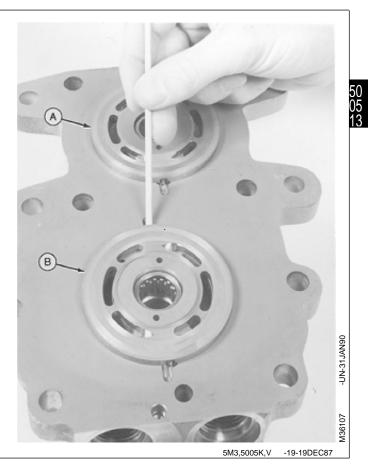
18. Inspect bearing plates. Bearing plates should be flat, free of all nicks, burrs, scratches and erosion around the ports. The bronze metal should show no scoring, smearing or be discolored.
