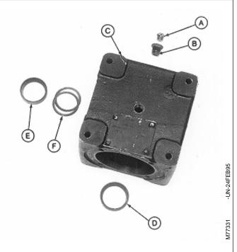
A—Vent Plug B—Adapter C—Gear Case D—Bearing Cup E—Bearing Cup F—Shims (as required)
