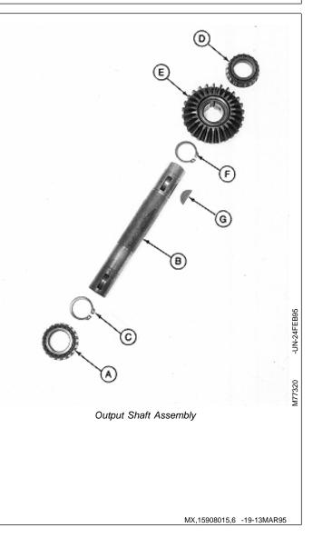
5. Install new bearing cup (F), if removed, using a driver set.
