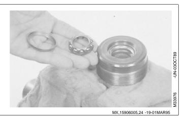
NOTE: Bearing cup is press-fit in bearing adjuster. Remove bearing cup only if replacement is necessary.
