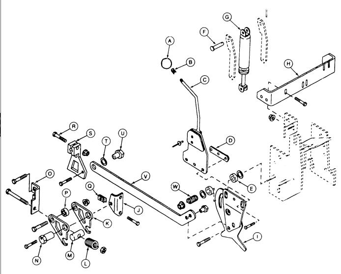
A—Knob B—Clip C—Speed Control Lever D—Weld Nut E—Friction Disc (2 used) F—Pin G—Torsional Dampener H—Bracket I—Control Plate J—Angle Bracket K—Detent Arm (2 used) L—Compression Spring
