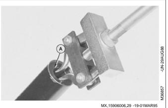
43. Remove nuts holding the four bolts to the fixture, and remove the bolts.
