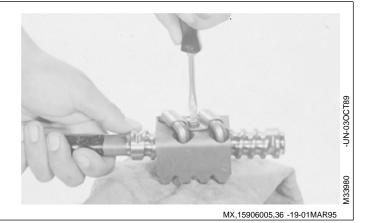
10. Pack upper worm bearing cone with multipurpose grease.
