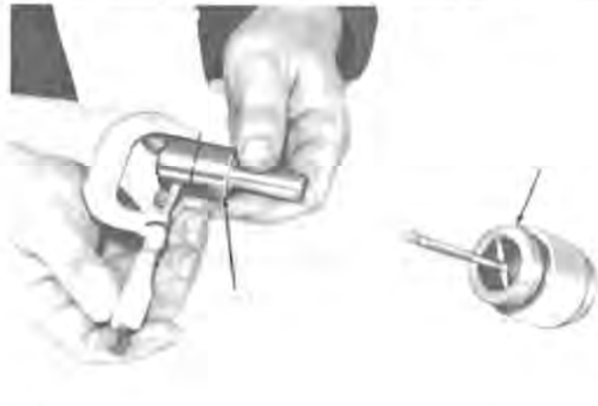
Fig. 15—Checking Variator Bearing and Shaft
