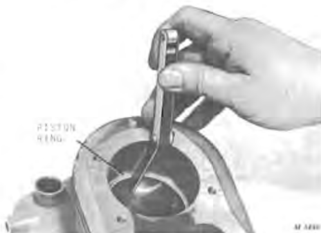
Fig. 30-Checking Ring End Gap
