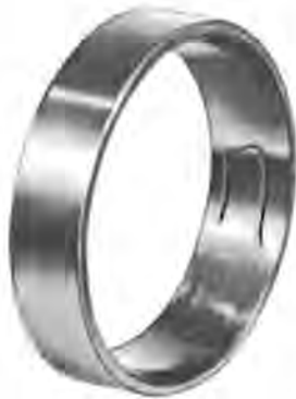
Fig. 26-Pitting and Longitudinal Crack
