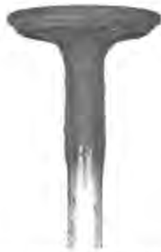
Fig. 5-Gummy Valve Causing Valve to Stick
