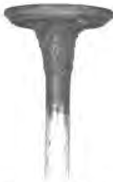
Fig. 2—Lead Deposits on Leaky Intake Valve
