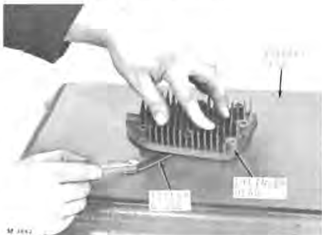
Fig. 9—Checking Surface of Cylinder Head
