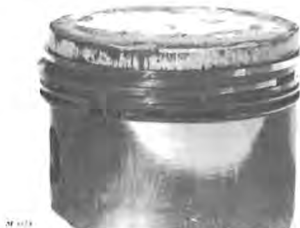
Fig. 8—Scored Piston and Rings Caused by Overheating as Temperatures Reach Melting Point of the Materials
