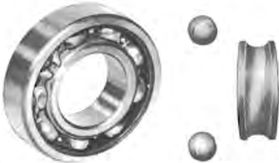
Fig. 27—Bearing Wear Caused by Misalignment
