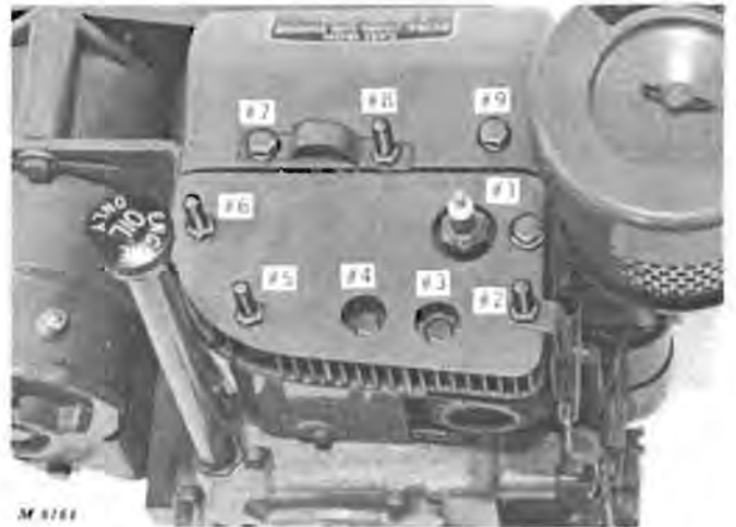
Fig. 25—Cylinder Head Bolt Tightening Sequence
