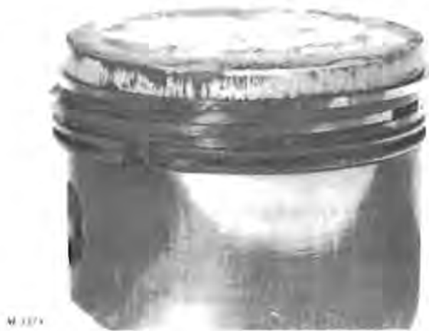
Fig. 6-Scored Piston and Rings Caused by Overheating as Temperatures Reach Melting Point of the Materials
