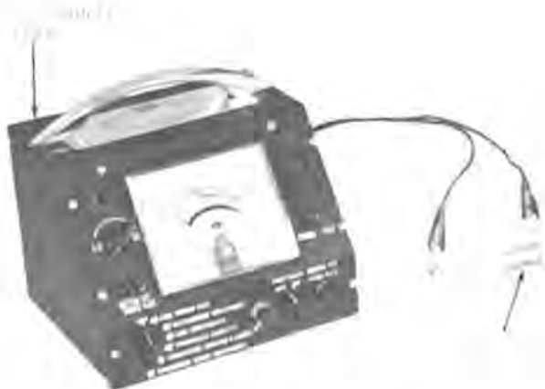
Fig. 13—Testing Condenser Capacity
