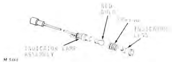
Fig. 5—Schematic View of Generator Indicator Lamp
