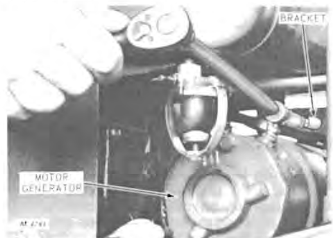
Fig. 34 - Adjusting Belt Tension on 112 Tractor
