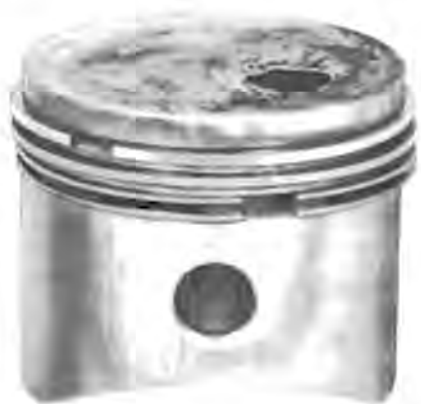
Fig. 17—Hole Burned in Piston Caused by Pre-Ignition
