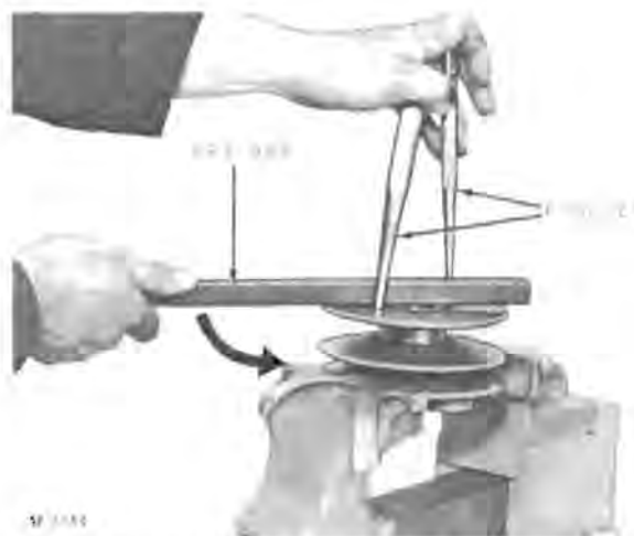
Fig. 12-Disassembling Center Variator Sheave
