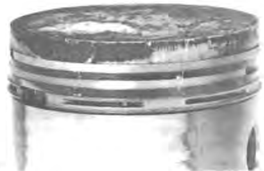
Fig. 16—Piston Top Land Burning Caused by Detonation
