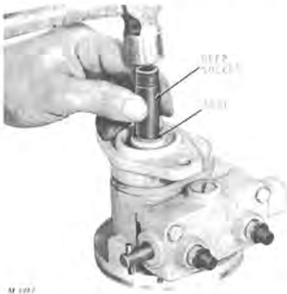
Fig. 19—Installing Shaft Seal
