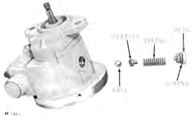
Fig. 20—Installing Relief Valve Assembly
