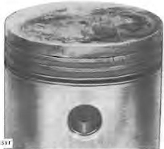
Fig. 11-Piston Rings Stuck and Broken Because of Lacquer, Varnish and Carbon Build-Up
