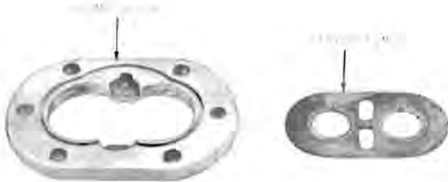
Fig. 5-Defective Pump Diaphragm and Pump Body
