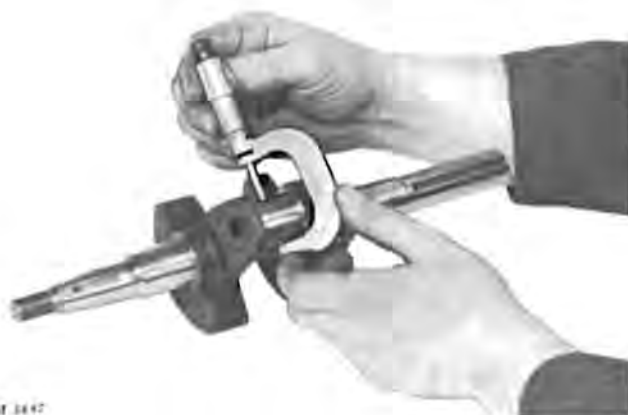
Fig. 20—Measuring Crankshaft Journal
