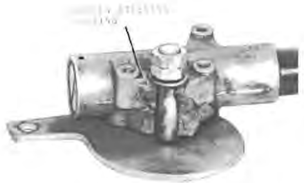
Fig. 4-Broken Steering Gear Housing
