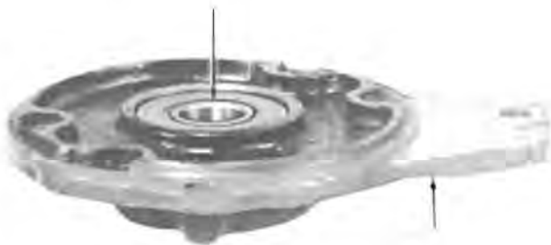
Fig. 20—Installing Bearing in End Frame
