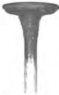
Fig. 2—Lead Deposits on Leaky Intake Valve
