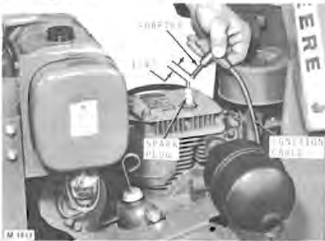
Fig. 2—Checking Spark at Plug
