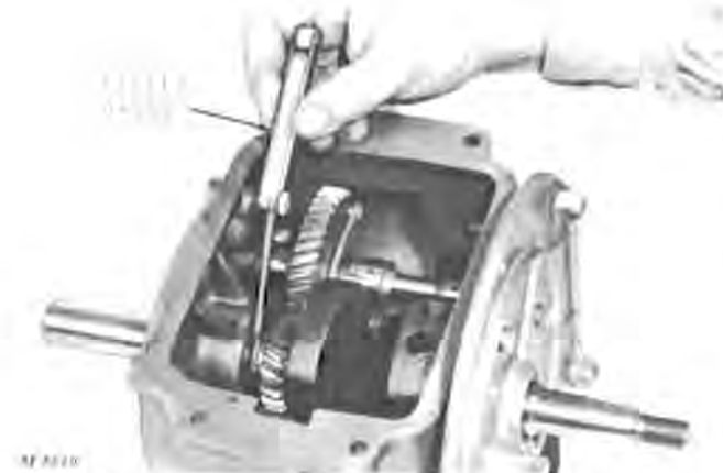
Fig. 33—Checking Crankshaft End Clearance
