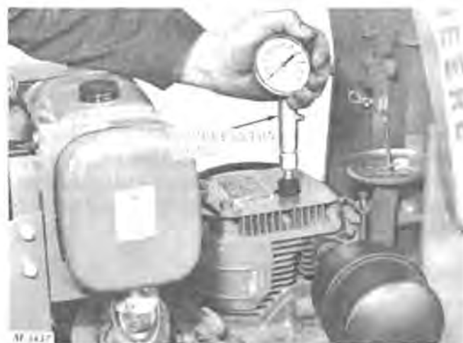
Fig. 8-Testing Engine Compression
