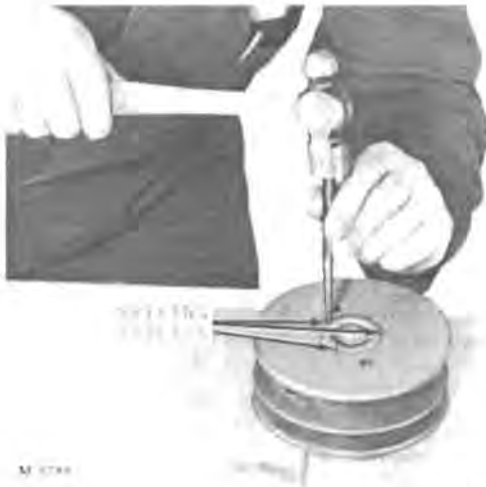
Fig. 18—Staking Variator Hub
