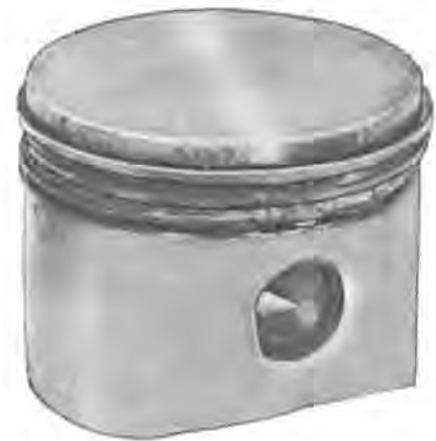
Fig. 21—Piston Damage Caused by Pin Lock Coming Loose
