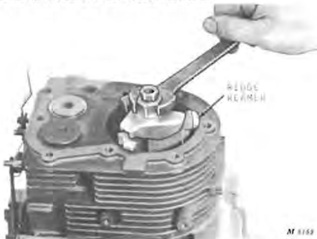
Fig. 3-Removing Ridge at Top of Cylinder Bore
