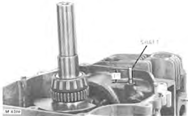
Fig. 11—Installing Governor Shaft
