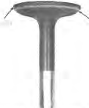
Fig. 4—Exhaust Valve Running Too Hot
