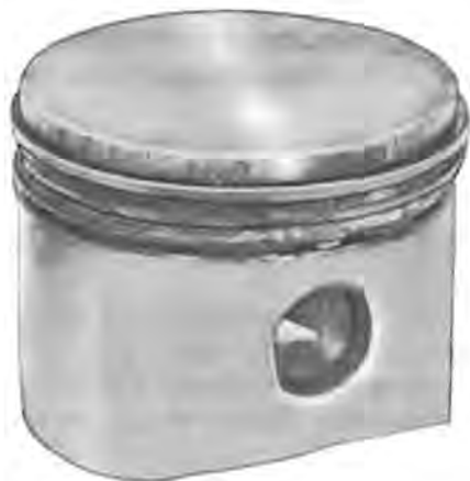
Fig. 19—Piston Damage Caused by Wrist Pin Lock Coming Loose
