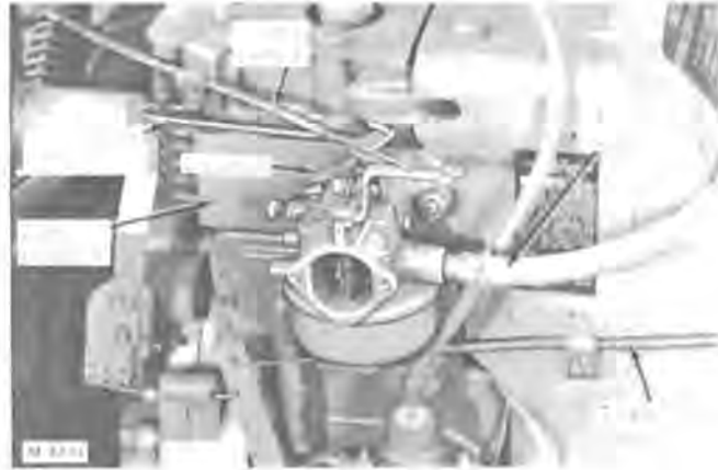
Fig. 21—Installing Carburetor Assembly on Cylinder Block (Air Cleaner Base Removed for Clarity)
