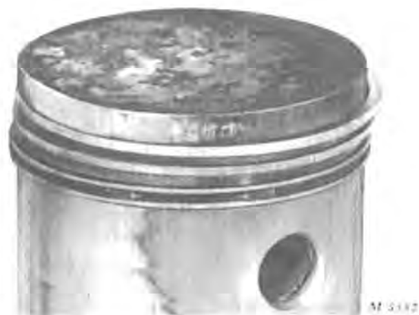
Fig. 10-Scratched Ring Faces Caused by Abrasives in the Engine
