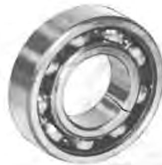
Fig. 25—Broken Races Caused by Misaligned Bearing During Installation
