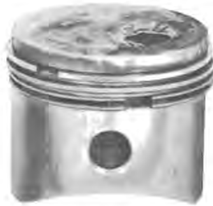
Fig. 19-Hole Burned in Piston Caused by Pre-Ignition
