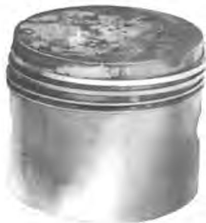
Fig. 18—Diagonal Piston Wear Pattern Caused by Bent or Twisted Connecting Rod
