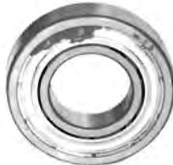
Fig. 29—Oil Seal Damage Caused by Careless Installation with Sharp Tool
