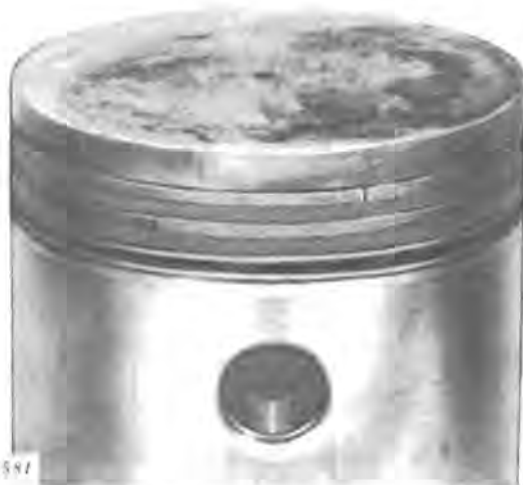
Fig. 9-Piston Rings Stuck and Broken Because of Lacquer, Varnish and Carbon Build-up
