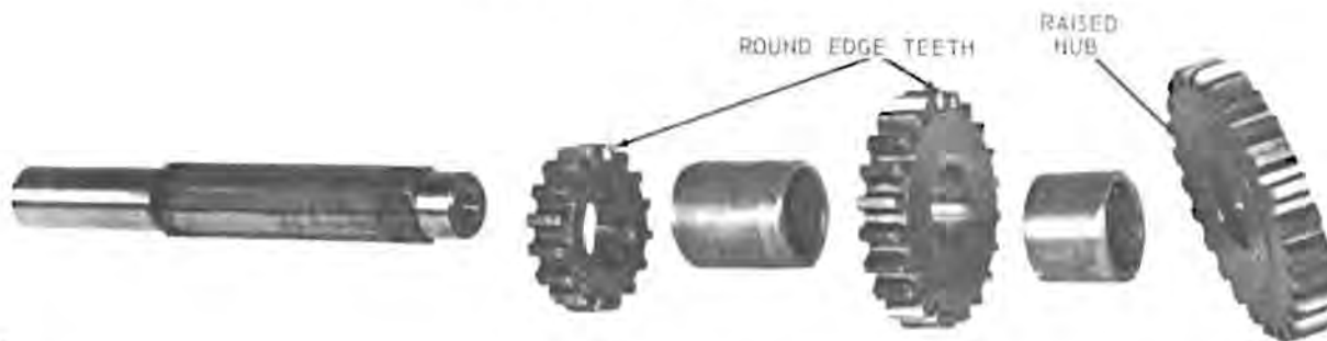
Fig. 26-Idler Shaft and Gear Assembly
