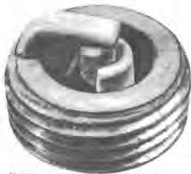
Fig. 8—Heat Shock Failure
