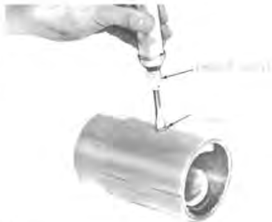
Fig. 22—Installing Field Coils
