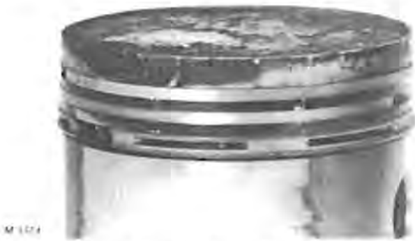
Fig. 18-Piston Top Land Burning Caused by Detonation
