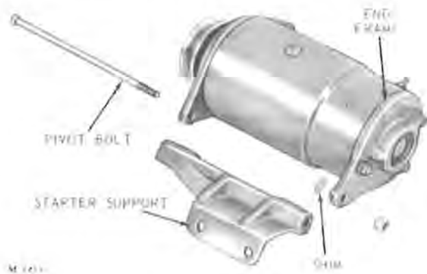
Fig. 31 - Add Shim Between End Frame and Support
