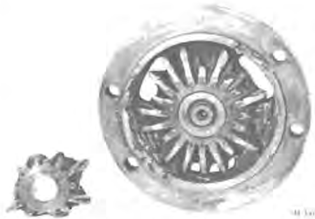
Fig. 22—Damaged Bevel Pinion Gears
