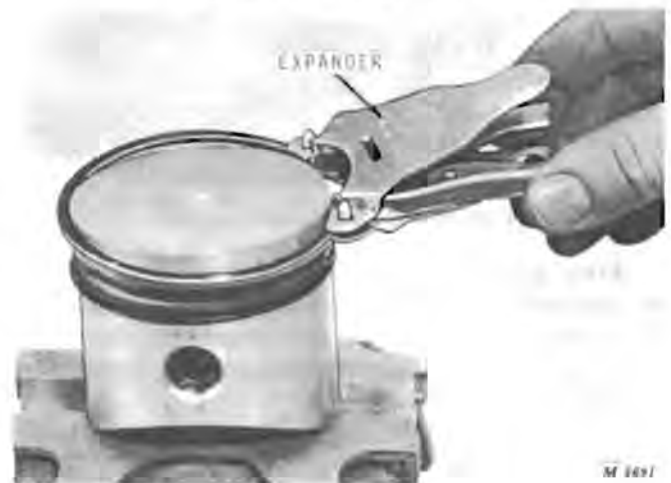
Fig. 37-Installing Rings
