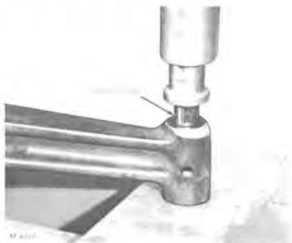
Fig. 7—Installing Axle Bushings
