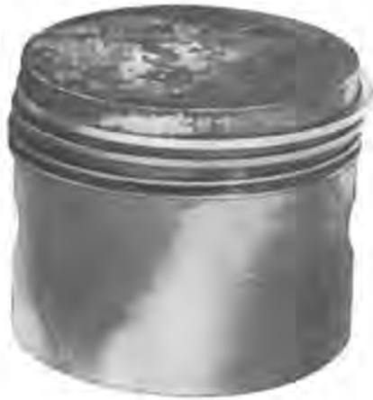
Fig. 20—Diagonal Piston Wear Pattern Caused by Bent or Twisted Connecting Rod
