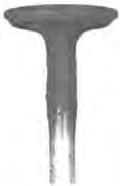
Fig. 5-Gummy Valve Causing Valve to Stick
