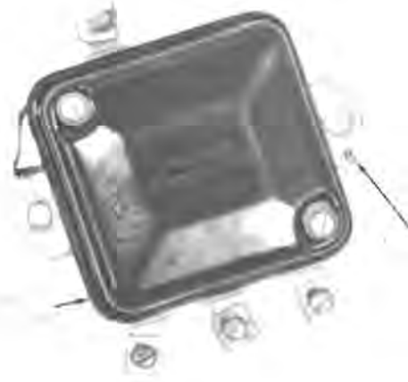
Fig. 29 - Letter "N" Indicates Negative Grounded Battery
