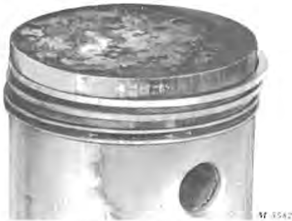
Fig. 12-Scratched Ring Faces Caused by Abrasives in the Engine
