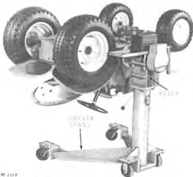
Fig. 9—Tractor Inverted on Repair Stand for Easy Transaxle Removal
