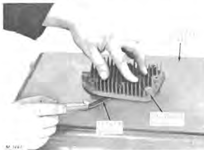
Fig. 9—Checking Cylinder Head Surface
