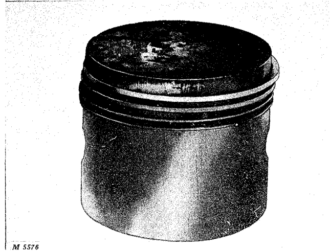
Fig. 20-Diagonal Piston Wear Pattern Caused by Bent or Twisted Connecting Rod
