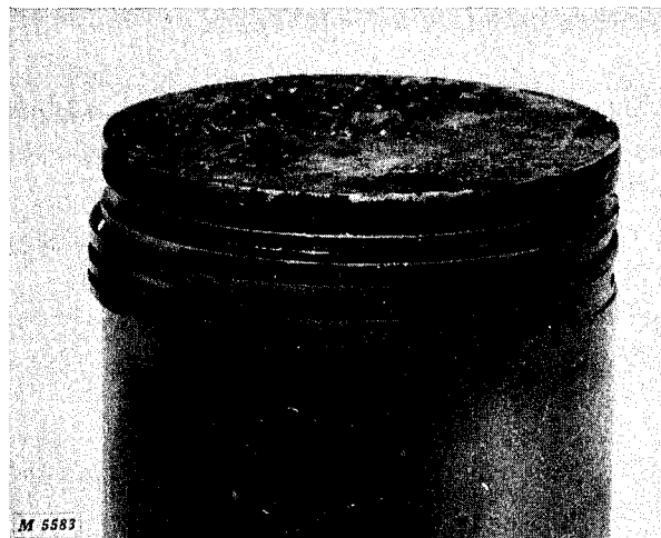
Fig. 14-Worn Oil Rings Which Cannot Provide Oil Control
