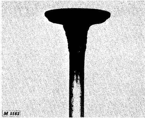
Fig. 2-Lead Deposits on Leaky Intake Valve
