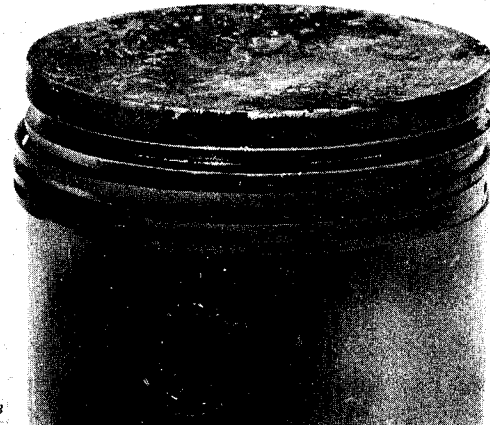
Fig. 13-Worn Oil Rings Which Cannot Provide Oil Control
