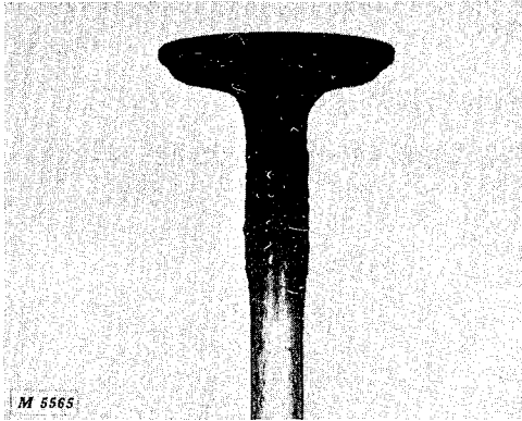
Fig. 5-Gummy Valve Causing Valve to Stick
