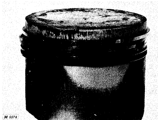
Fig. 8-Scored Piston and Rings caused by Overheating as Temperatures Reach Melting Point of the Materials
