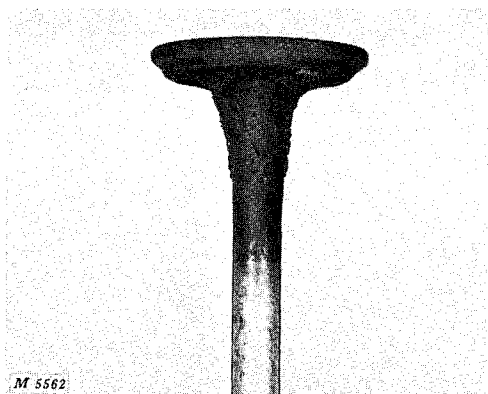
Fig. 2-Lead Deposits on Leaky Intake Valve
