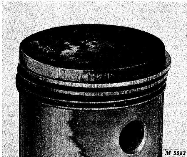
Fig. 13-Scratched Ring Faces Caused by Abrasives in the Engine
