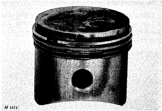
Fig. 19-Hole Burned in Piston Caused by Pre-Ignition
