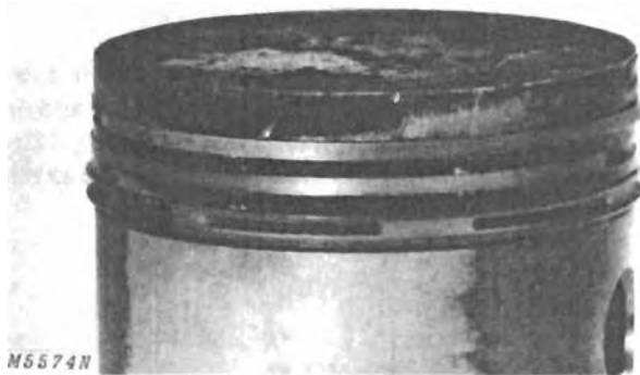
Fig. 19-Piston Top Land Burning Caused by Detonation
