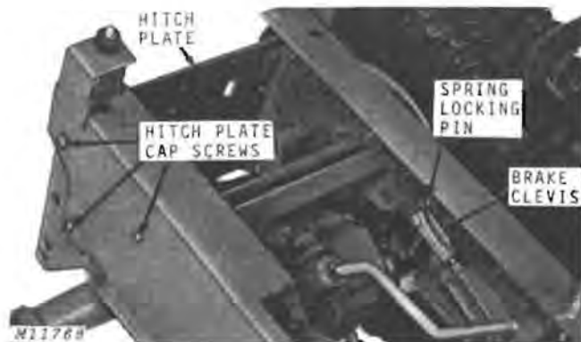
Fig. 9-Preparing Transaxle for Removal (Right Rear Wheel Removed for Clarity)
