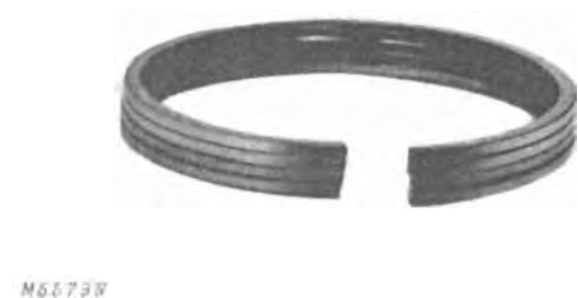
Fig. 10-Piston Rings with Improper End Gap
