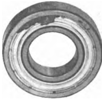
Fig. 32-Oil Seal Damage Caused by Careless Installation with Sharp Tool
