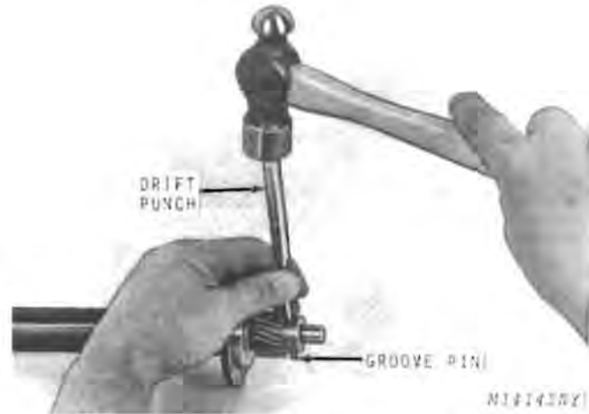
Fig. 10-Removing Gear From Actuator Shaft
