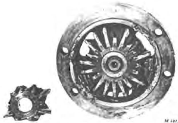
Fig. 20-Damaged Bevel Pinion Gears
