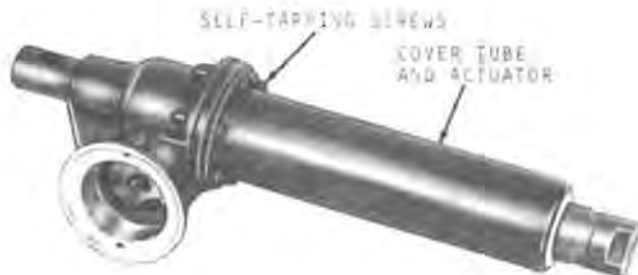
Fig. 13-Installing Actuator Assembly to Gear Box
