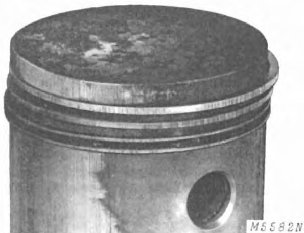
Fig. 13-Scratched Ring Faces Caused by Abrasives in the Engine
