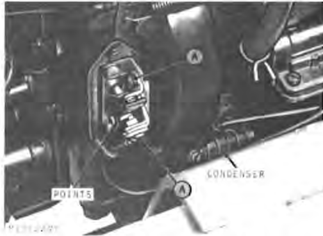
Fig. 12-Replacing Breaker Points and Condenser
