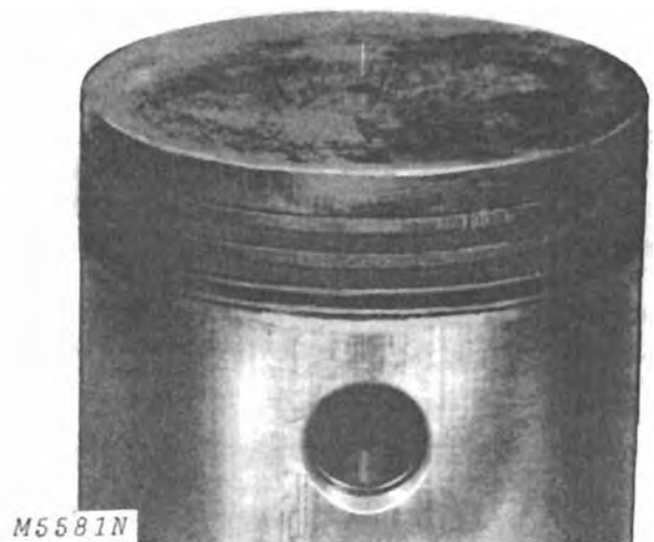
Fig. 12-Piston Rings Stuck and Broken Because of Lacquer, Varnish and Carbon Build-Up
