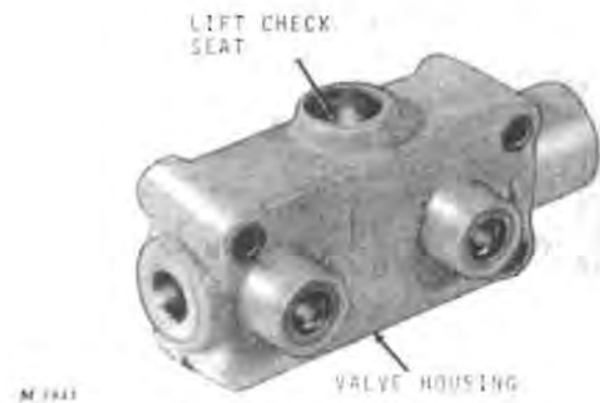
Fig. 9-Checking Valve Housing for Wear and Damage
