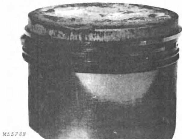
Fig. 9-Scored Piston and Rings
