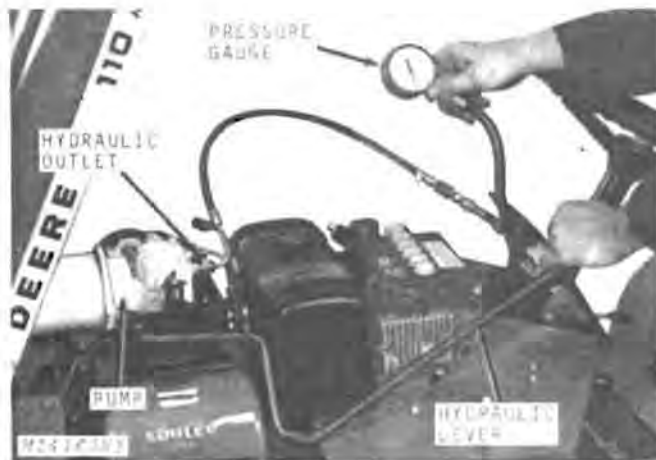
Fig. 7-Pressure Gauge Installed on Valve
