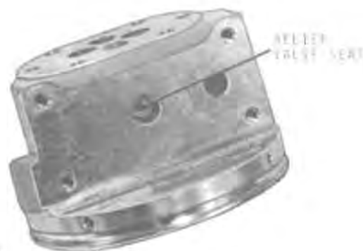
Fig. 6-Removing Relief Valve Seat
