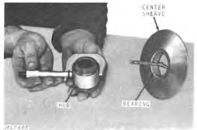
Fig. 22-Checking Center Sheave Bearing and Hub
