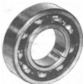
Fig. 28-Broken Races Caused by Misaligned Bearing During Installation
