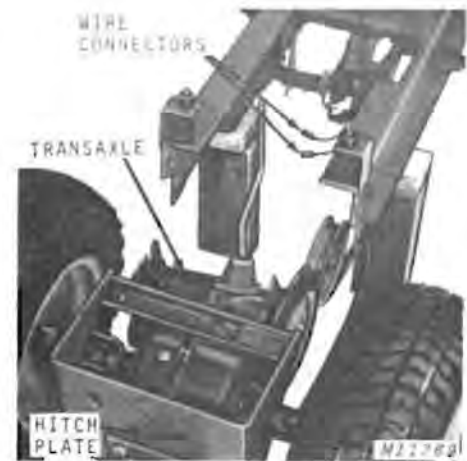
Fig. 10-Hitch Plate and Transaxle Assembly Removed from Tractor
