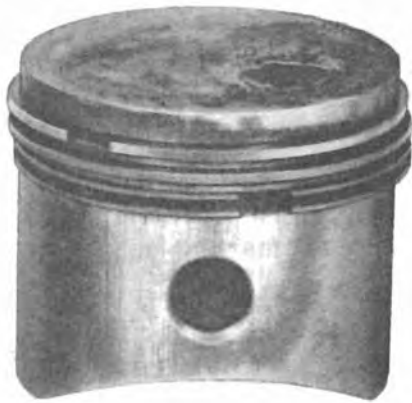
Fig. 21-Hole Burned in Piston Caused by Pre-Ignition
