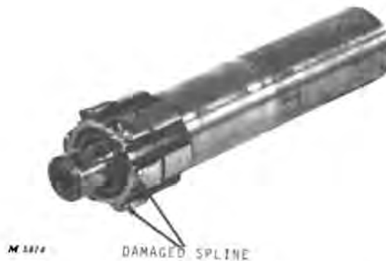
Fig. 21-Damaged Input Shaft Spline
