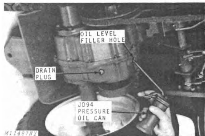
Fig. 3-Adding Oil to Transaxle
