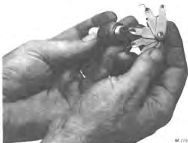
Fig. 10-Checking Spark Plug Gap
