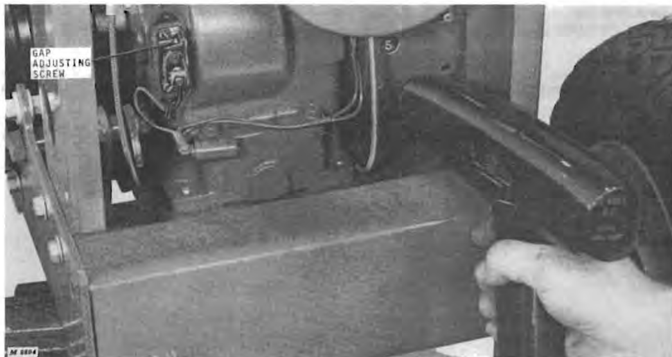
Fig. 15-Timing Ignition with Timing Light
