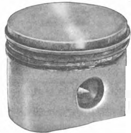
Fig. 22-Piston Damage Caused by Piston Pin Retainer Coming Loose
