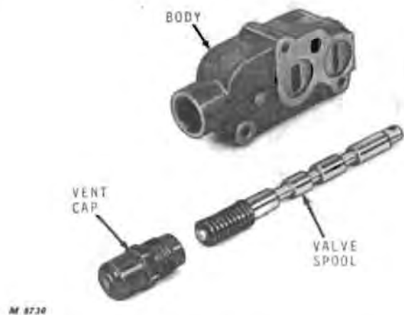
Fig. 6-Removing Valve Spool from Valve Body
