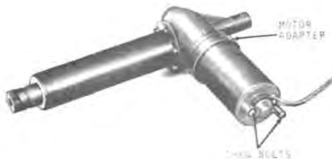
Fig. 5-Removing Drive Motor From Actuator
