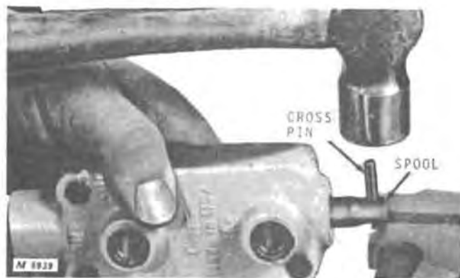
Fig. 14-Installing Cross Pin in Spool
