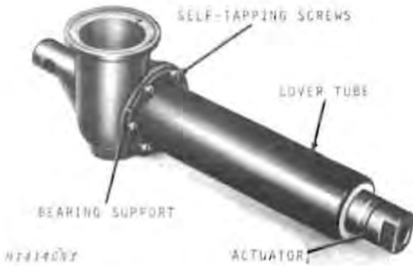
Fig. 8-Removing Cover Tube and Bearing Support
