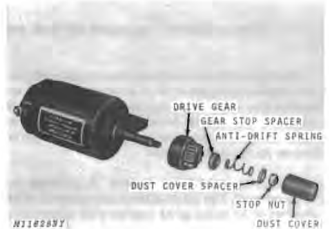
Fig. 17—Disassembling Starter Drive
