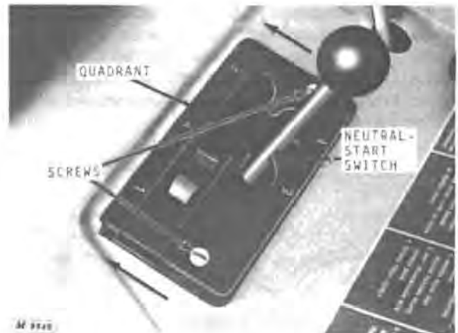
Fig. 8-Adjusting Quadrant Neutral-Start Switch
