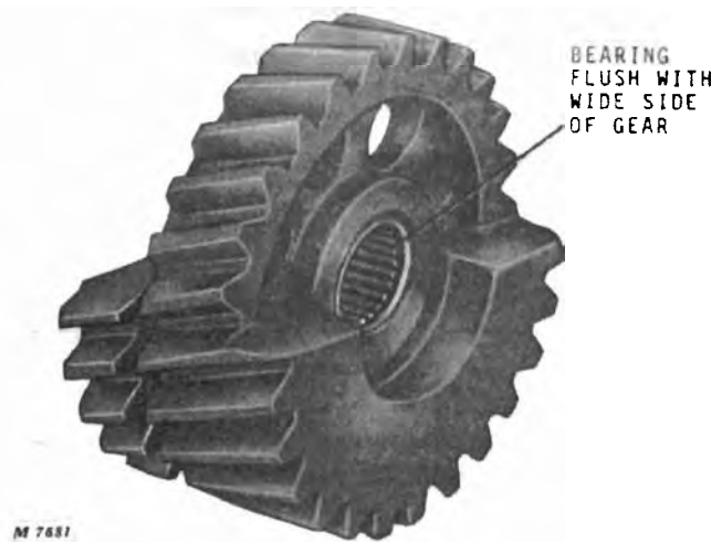
Fig. 7-Installing Needle Bearing in Gear
