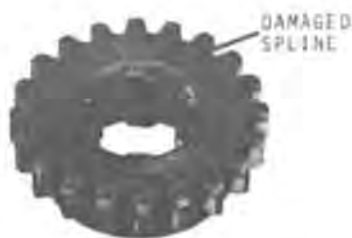
Fig. 22-Worn Spline in Shifter Gear
