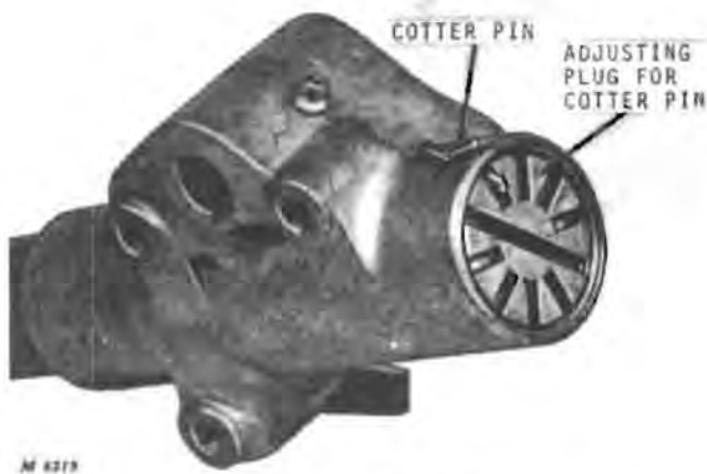
Fig. 13-Cotter Pin Through Housing
