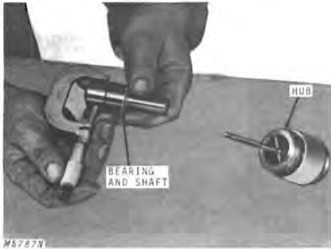
Fig. 23-Checking Variator Bearing and Hub
