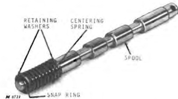
Fig. 7-Removing Spool Centering Spring
