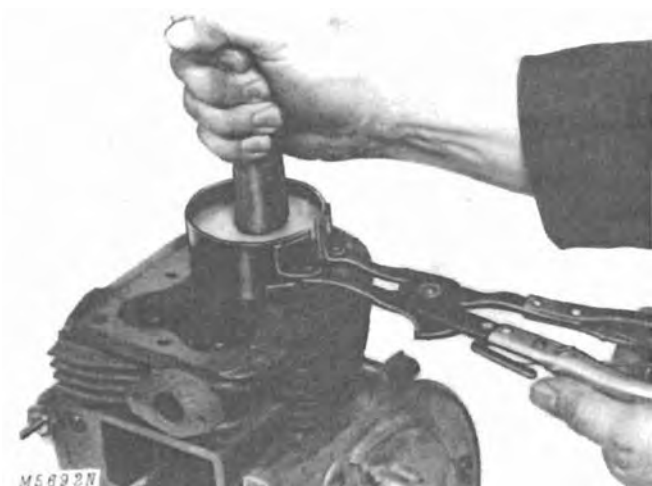
Fig. 47-Installing Piston in Cylinder
