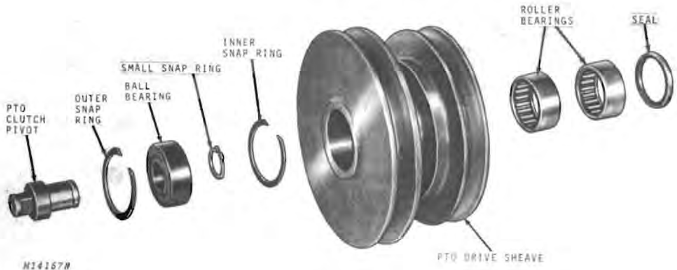
Fig. 1-PTO Clutch Drive Sheave Assembly
