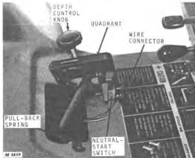
Fig. 49-Connecting Plunger-Type Neutral-Start Switch
