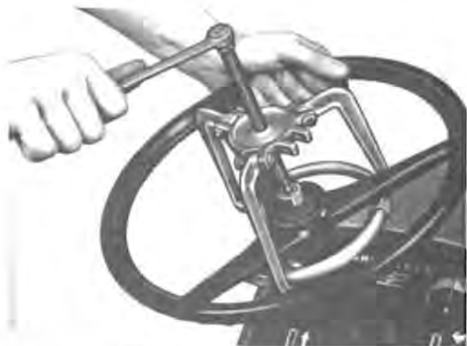
Fig. 9 Removing Steering Wheel
