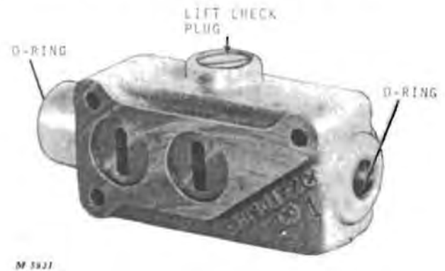
Fig. 8-Removing O-Rings and Lift Check Assembly
