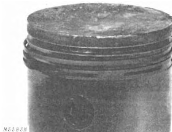
Fig. 14-Worn Oil Rings Which Cannot Provide Oil Control
