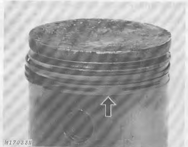
Fig. 12-Worn Oil Rings Which Cannot Provide Oil Control
