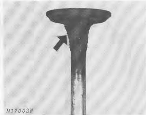
Fig. 5-Lead Deposits on Leaky Intake Valve
