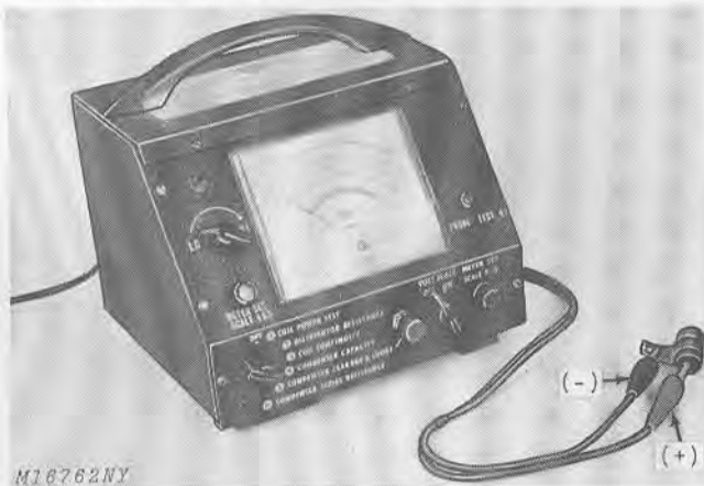
Fig. 16—Testing Condenser Capacity
